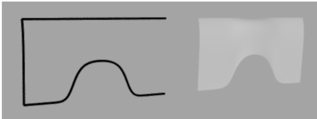
Figure 16: Birail1 Object (left: Curves, right: Resulting Swept Surface)
