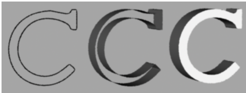
Figure 13: Extrude Object (left: Curve, middle: normal Extrusion, right: Extrusion with Caps)
