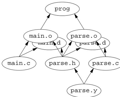
The vertexes and edges for the include file dependency files are also present as these are important for *make* to function correctly.
