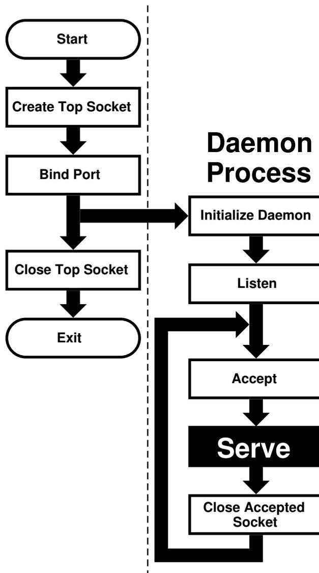
This flowchart is good for *sequential servers*, i.e., servers that can serve one client at a time, just as we were able to with our *daytime* server. This is only possible whenever there is no real “conversation” going on between the client and the server: As soon as the server detects a connection to the client, it sends out some data and closes the
