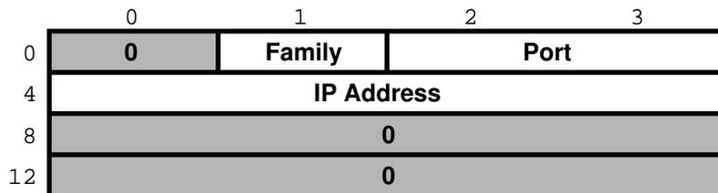
The three important fields are `sin_family`, which is byte 1 of the structure, `sin_port`, a 16-bit value found in bytes 2 and 3, and `sin_addr`, a 32-bit integer representation of the IP address, stored in bytes 4-7.
