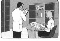
lysis on a lab form and punch it on paper tape. At this point, a lab technician examines the printed analysis and transmits the taped data to Teletype sets within the shop. This new system has reduced the time for analyzing production run samples to about two minutes per sample.
