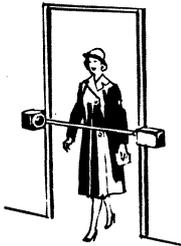
**RELAY KIT ONLY.** Now you can build your own ultra-sensitive photoelectric relay at very low cost. It's fun to build—and you'll find dozens of uses for it in automatic control of lights, door openers, burglar alarms, counting devices, etc. Ideal for turning on house or store lighting each evening at dusk—turns itself off at dawn.
