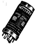
For use in filter circuits, audio by-pass circuits and TV applications. Capacitors feature complete stability under heavy ripple current, high surge voltages and high temperatures. Units are encased in compact, rubber-sealed aluminum cases. FP types have the exclusive Mallory Fabricated Plates—anoles specially constructed of metalized cotton gauze. WP types have etched-plate anodes. PFP and PWP types are identical in performance to FP
