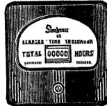
120-Volt Type. Elapsed time panel meters for keeping life and performance records based on operating time. Self-starting synchronous clock motor. Counter indicates up to 9999.9 hours, then recycles to 0. Matches Simpson standard  $3\frac{1}{2}$ " meters exactly in panel appearance. Flange size,  $3\frac{1}{8} \times 3\frac{3}{8}$ "; body diameter,  $2\frac{3}{4}$ "; body depth,  $2\frac{1}{8}$ ". For 120 v., 60 cycle AC. Shpg. wt., 2 lbs.
