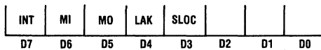
Figure 3. Left/Right Port Status Register (CR1) (If C urrent Port = Left/Right, Then O pposite Port = Right/Left)
