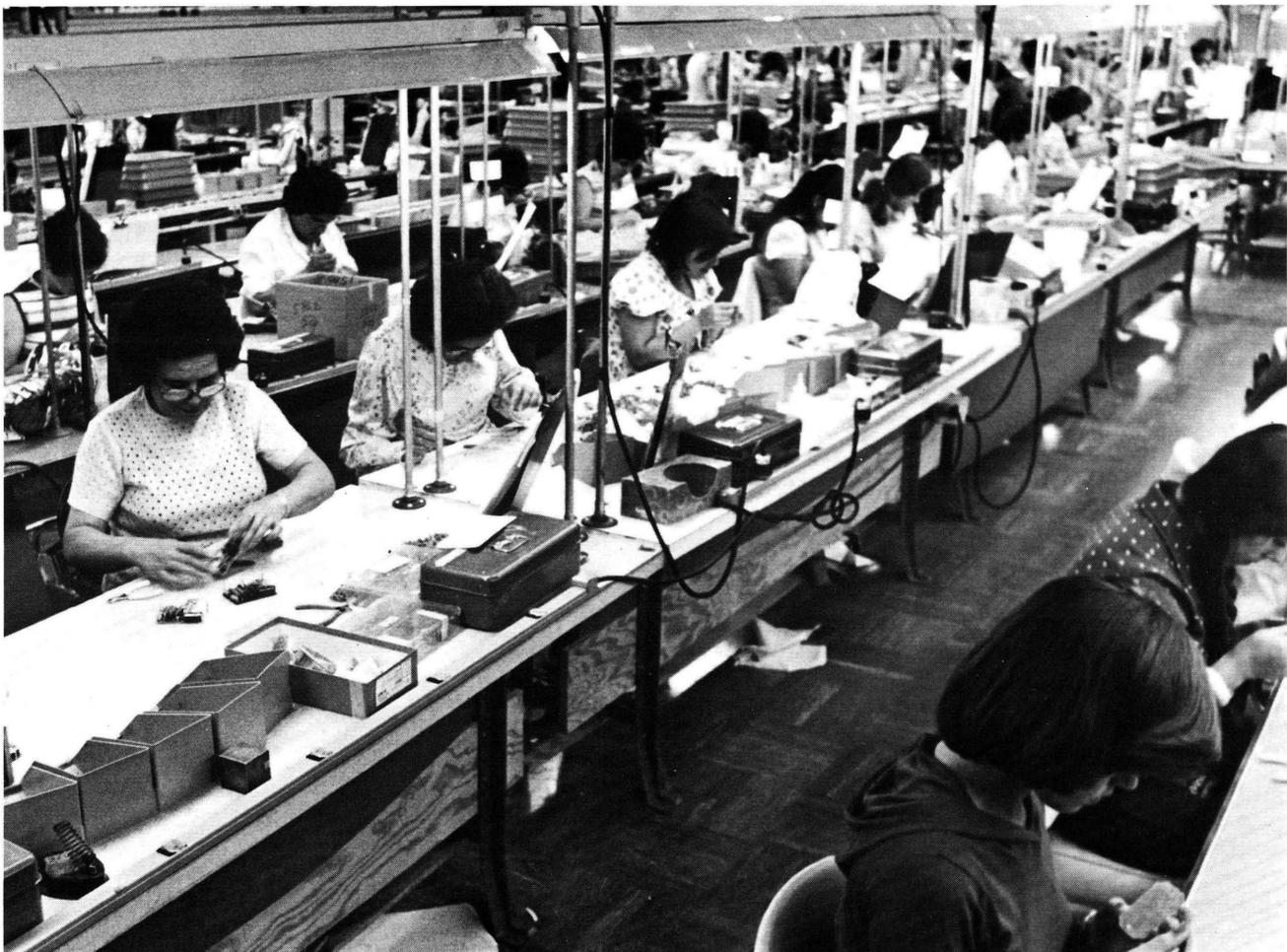
*High volume burn-in test stations assure reliable digital panel meters at an economical cost.*
