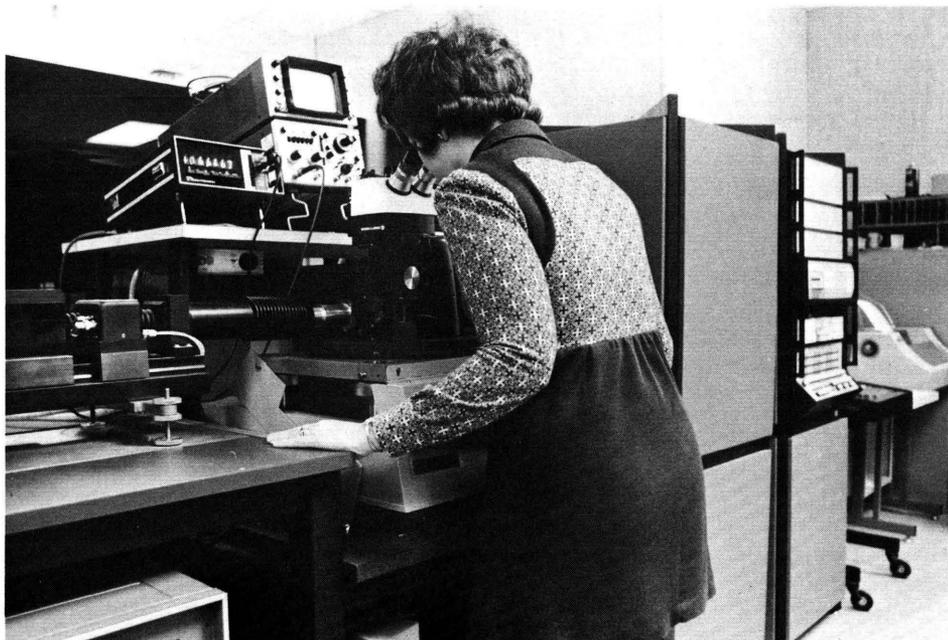
*Our proprietary thin-film-on-silicon trimming process allows precise tailoring of integrated circuit element values prior to final encapsulation. Computerized laser trimming of our IC multipliers, op amps, and converters enhances their accuracy, but decreases their cost.*
