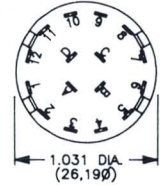
TERM. NOS. MOLDED ON HOUSING
