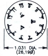
TERM. NOS. MOLDED ON HOUSING
