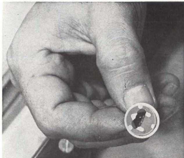
Light-actuated semiconductor analog of the mechanically operated potentiometer (left) is being tested for effects of temperature on voltage deviations by Guido Galli of Giannini Controls
