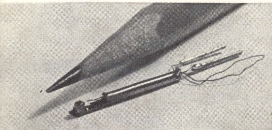
Detector can be inserted in body cavities as radioisotope tracer
