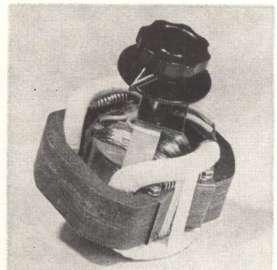
S.E.I.M. brushless transformer varies output by changing angle of secondary winding
