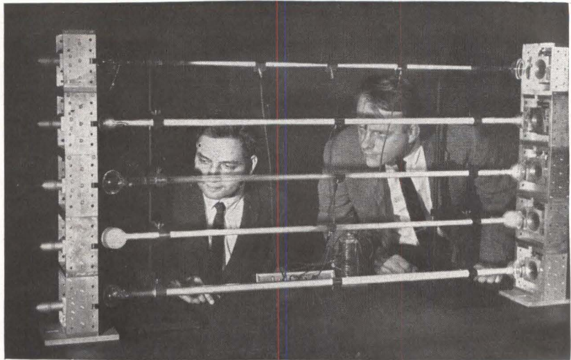
LASER TUBES containing the five noble gases are checked for alignment
