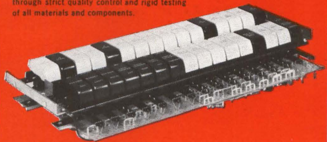
Photos of Lowery tonal effect selector show Panelyte sheet functioning as insulator and support for moving and fixed contacts of multi-pull electrical switches.
