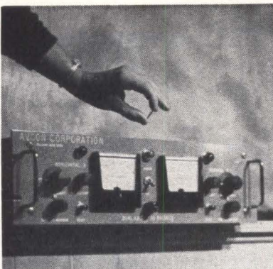
POWER SUPPLY used with electrolytic cells to accomplish gyro balance
