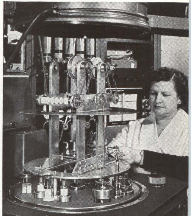
Interior of a special high-vacuum unit showing a special developed fixture used in coating thin-film substrates.
