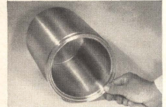
OFHC COPPER A housing that has been backward extruded and machined. Note solid end.
