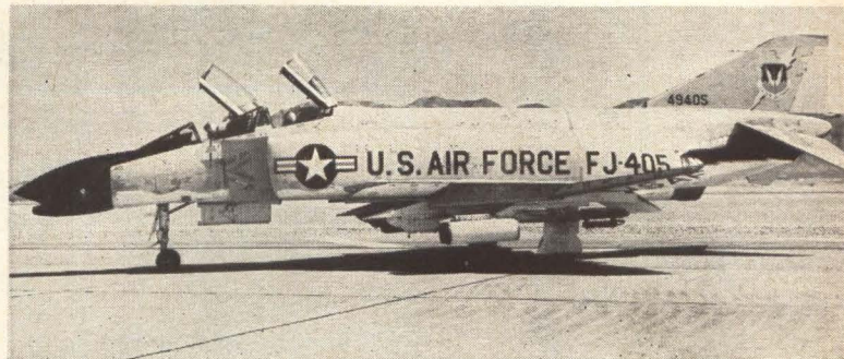
McDonnell RF-4C Phantom II will become a major electronic reconnaissance plane for the Air Force. Its top speed exceeds 1,400 miles an hour. Later on, the Navy will probably go to the Grumman EA-6A Intruder.
