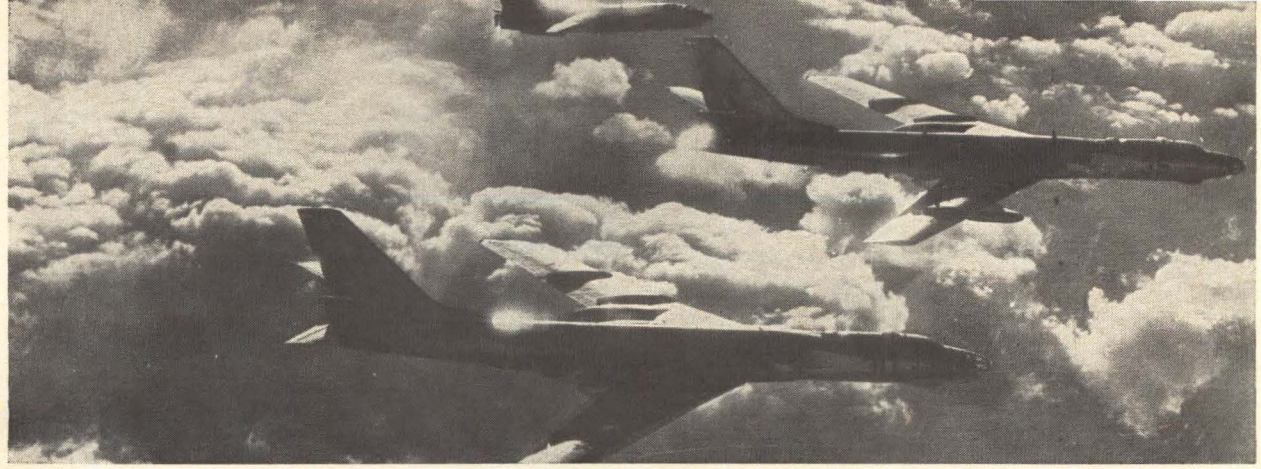
Action in the North Pacific. Two Soviet Badger reconnaissance bombers that flew over the attack carrier Kitty Hawk (CVA-63) are escorted away by a Navy F-4 Phantom II (not shown) and an F-8 Crusader. The twin-jet Badger is used by both the Soviet Navy and Air Force. Its official name is the Tupolev TU-16. It has a 3,975-mile range.
