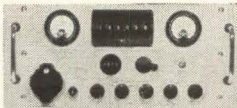
CSG Series . . . 136-138 mc in 1kc steps, 400-406 mc in 1kc steps, 1700-1710 mc in 10kc steps.
