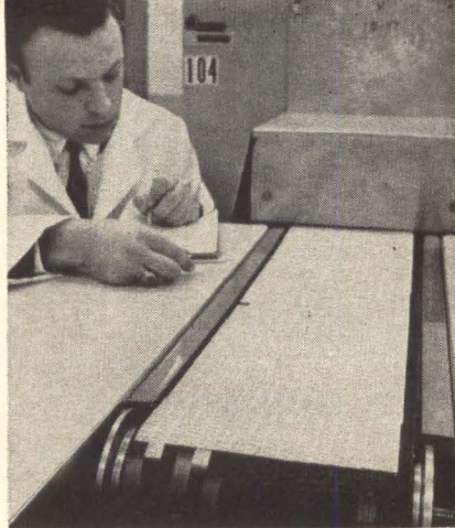
Passive elements are screened on ceramic wafers and baked.
