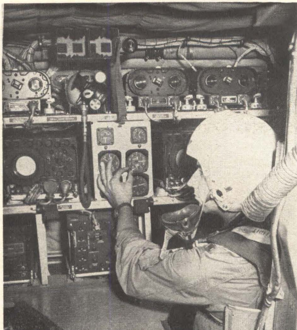
Raven position No. 2—there are four. The officer is correcting the altimeter reading on his instrument-panel repeater. The repeater panel, sandwiched neatly between two ALA-6's contains a compass, air-speed indicator, altimeter, cabin-pressure indicator, clock and latitude-longitude indicator. Bottom row contains another APR-14 and APR-8B. Top row holds three ANH-2 wire recorders, the AIC-10 interphone control panel, and an emergency oxygen bottle. Newer gear performs the annotation function automatically.
