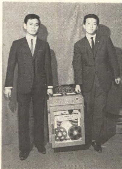
Lighter load. A switch to IC's for the logic circuits slashed the size and weight of Fujitsu's Fanuc 260 NC unit.
