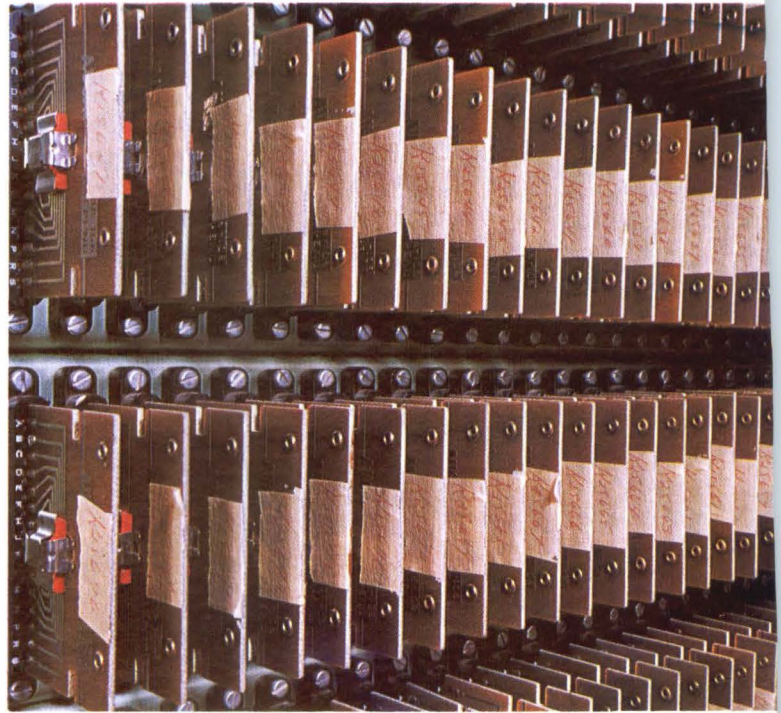
IC's for the Apollo program are operated in Raytheon's burn-in rack for 168 hours. The devices are subjected to power and input signal stresses that simulate actual use as they perform in an 8-volt ring oscillator.
