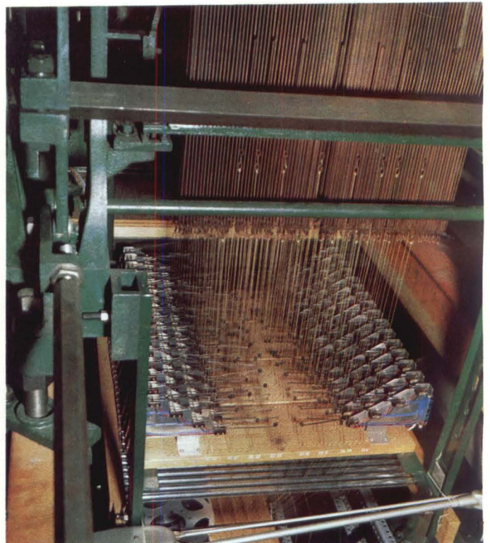
Feedback switches detect any faulty operation of the selection or lift mechanism. The actuators are at the top, with the selectors hanging down below them. The black bead on each selector operates one of the small snap-action switches if that selector is raised. At the completion of the lift motion, the switch settings are compared with the instructions from the paper tape reader. If they don't match, the selection operation is repeated. A few of the beads are just visible peeping over the edge of the platform in the photograph on page 93.
