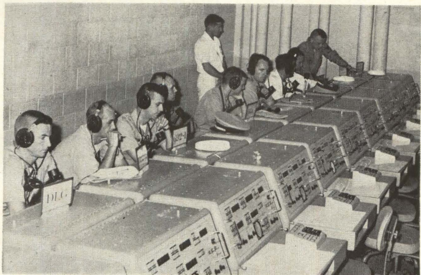
At the helm. Students operating these consoles "maneuver" ships on the gameboard sea after getting commands from CIC mockups.
