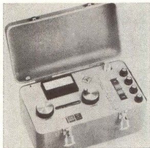
Manual balance digital indicator MDX-11 is used with bonded strain gage force and pressure transducers with 2 mv/v or 3 mv/v output signals. Full scale output is 100,000 counts with a 30% overrange capability. A course control knob of 12 add-to steps of 10,000 counts each is included. Accuracy is 0.05%. Transducers Inc., E. Rivera Rd., Santa Fe Springs, Calif. [366]
