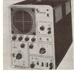
Triggered sweep, 5-in. oscilloscope/vectorscope T0-50 offers features normally found only in lab-quality test instruments at a price of $329.50. Features include 10-Mhz bandwidth; d-c amplifiers to eliminate pattern bounce, permit viewing a-c and d-c simultaneously; and calibrated vertical attenuator and horizontal time base. Lectrotech Inc., 4529 N. Kedzie Ave., Chicago [368]
