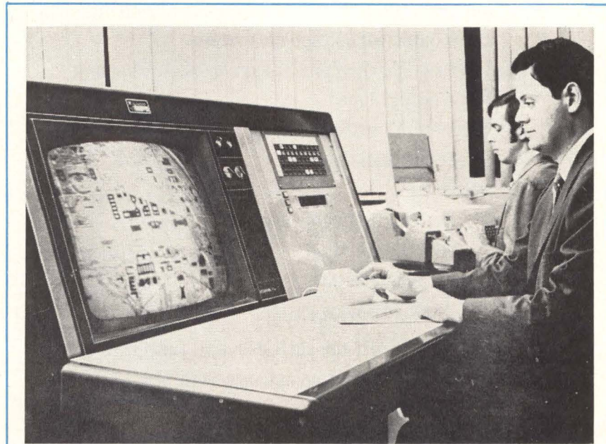
Making the scene. With New York City's police "war room" already operating—direct phone links to precincts, tv at likely trouble spots, and a small computer—Sylvania is field testing this computerized dispatch system with other police departments. It's aimed at getting police to where they're needed quickly. The Sylvania approach is called automated command control and dispatch. When a crime or accident is reported, a clerk types the location on the computer console, keying in a priority code indicating the seriousness of the situation. In seconds, the computer displays a letter symbol at that location on the dispatch monitor, a cathode-ray tube. Simultaneously, patrol units assigned to the area are indicated on the crt; a color code indicates the availability of the units. The dispatcher then selects a unit, assigns it by radio to where it's needed, and feeds this information to the computer, which displays the assigned unit on the monitor.
