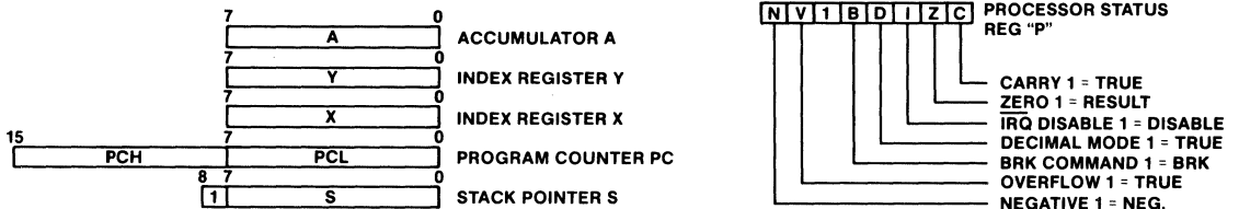
Figure 3. Microprocessor Programming Model
