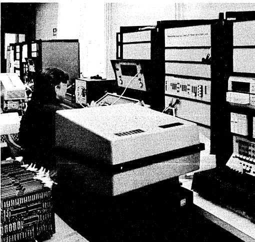
Figure 6. A Teradyne Test System Utilized in SBC 80 Board Testing
