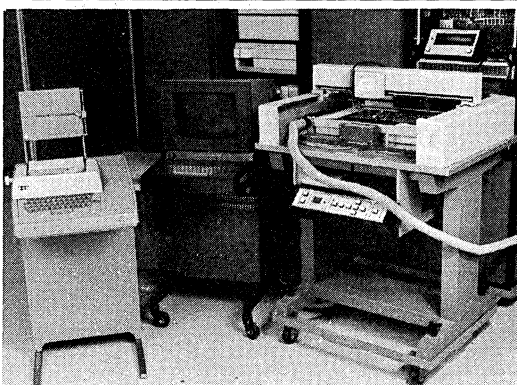
Figure 6. A Teradyne Test System Utilized in iSBC 86/12A™ Board Testing
