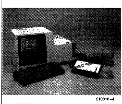
210818-4 Figure 1. A typical 8042 Development Configuration. The host system is an Intellec Series IV. The ICE-42 module is connected to a user prototype system.
