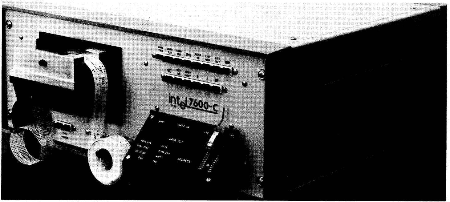
Fig. 1. Photograph of ROM Programmer Using MCS-4
