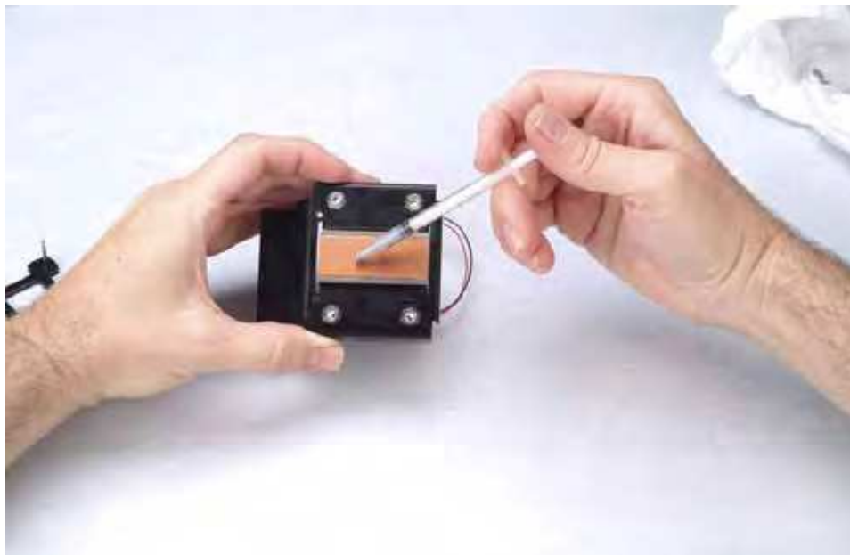
Figure 8. Applying the Thermal Grease
