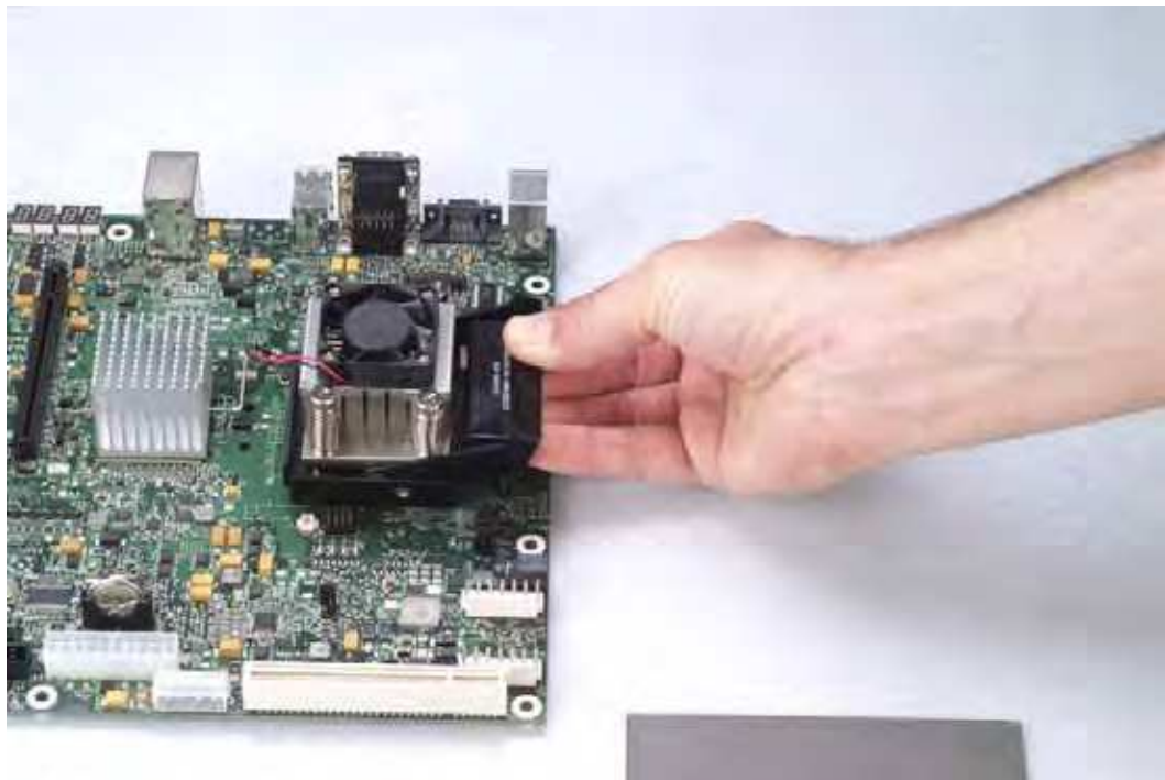
Figure 10. Installing the Heatsink
