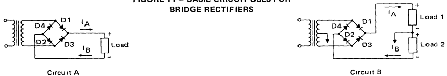
FIGURE 11 – BASIC CIRCUIT USES FOR BRIDGE RECTIFIERS
