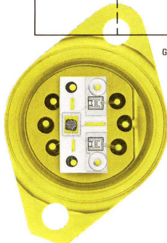
Dual power driver demonstrates hybrid device capability. This off-the-shelf device, type MCH2890R, provides a 6-ampere output for driving mechanical loads.
