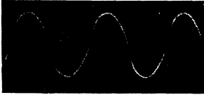
Fig. 20(a) - CA3070 terminal No. 6, oscillator waveform 1.1 V p-p 3.58 MHz.
