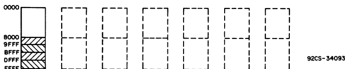
1-kilobyte and 2-kilobyte segments between F000 and FFFF can be inhibited similarly as shown under 2(b).
