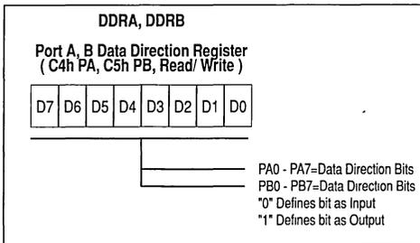
**Figure 24. I/O Port Option Registers**
