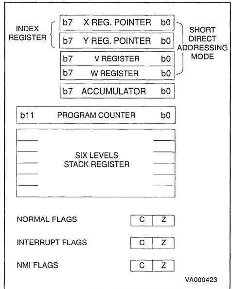
**Figure 3. ST62xx Core Block Diagram**
