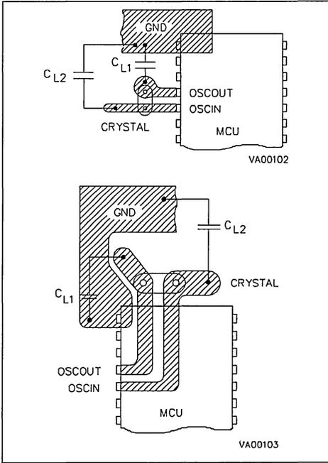
The reduction of inductance can be obtained by making the lengths and surfaces of the track smaller. This can be obtained by placing the track loops closer on the same PCB layer or on top of one another (Figure 2). The resulting loop area is small and the electromagnetic fields reduce one another.
