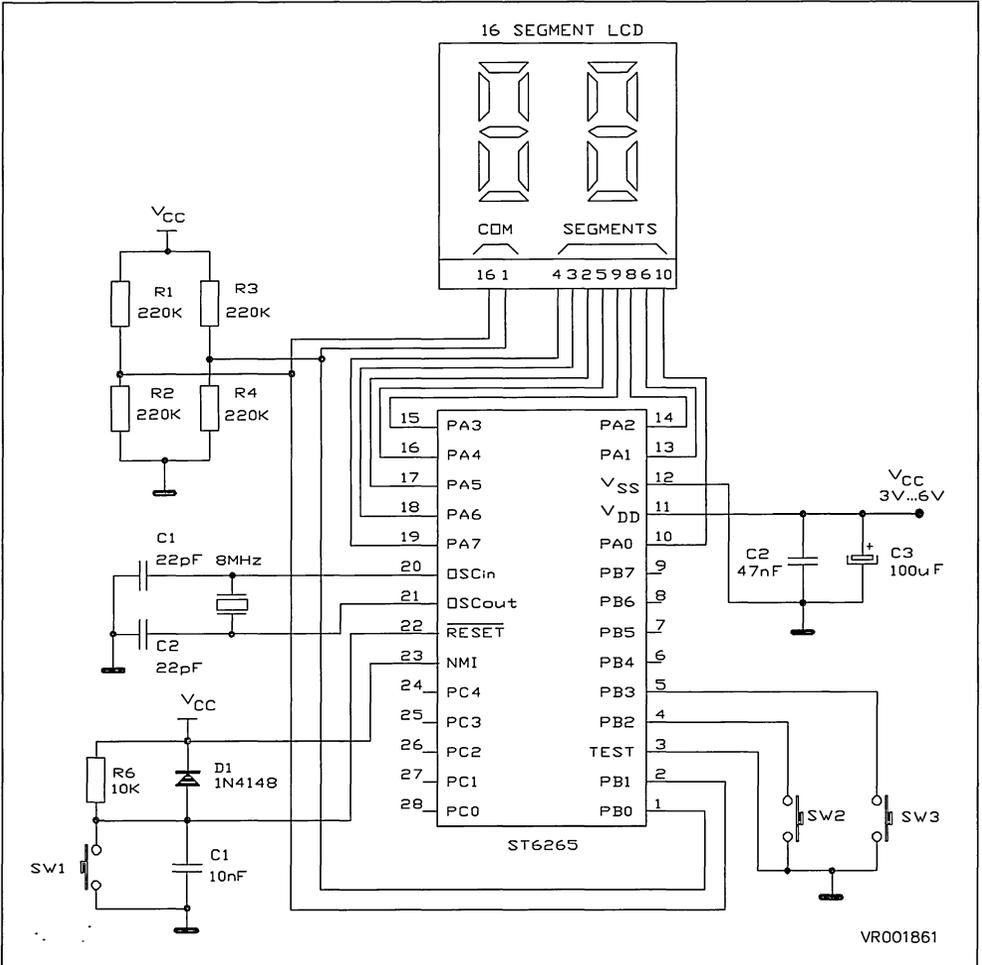
The software for the LCD display operates in interrupt mode, driving I/O pins by the CPU at instants defined by the Timer1 interrupts. When the LCD drive tasks are finished, the main application program can continue.
