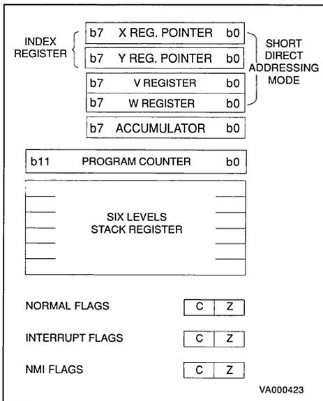
Figure 3. ST62xx Core Block Diagram
