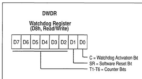
Figure 32. Digital Watchdog Block Diagram
