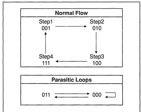
The trace points can be used also to control the flow of the tasks. In such a case, a "called" task can be only called by a "calling" task. Such checks can be done at the beginning and at the end of each task.
