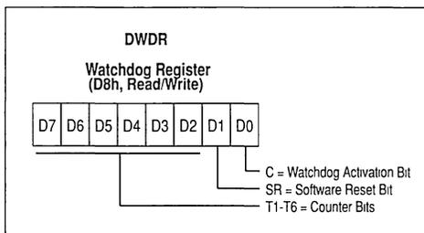
Figure 31. Digital Watchdog Block Diagram
