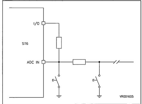
**Figure 4. Keyboard reading**
