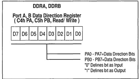
**Figure 25. I/O Port Option Registers**
