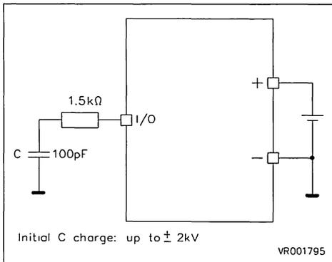
overvoltage higher than the maximum specified rating is applied on the supply pins. For the second test, a high current pulse is injected in I/O pins of a device supplied normally. In both tests, latch-up is
