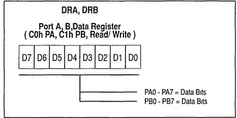
**Figure 24. I/O Port Data Direction Registers**
