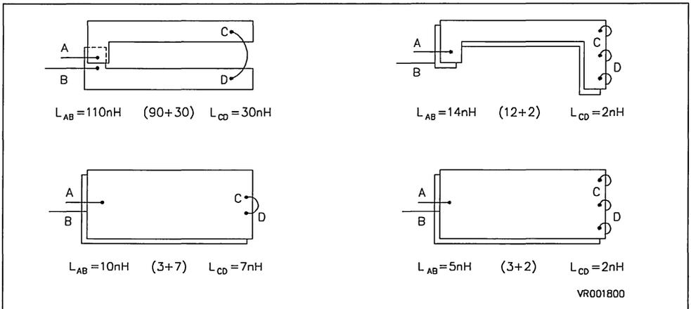
Note: This test is done with a double sided PCB. Insulator thickness is 1.5mm, copper thickness is 0.13mm. The overall board size is 65 x 200mm.
