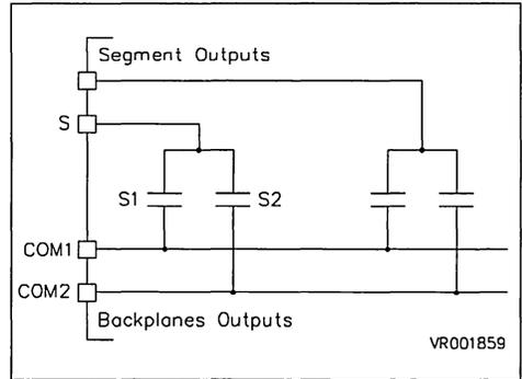
Figure 4. LCD Signals for Duplexed Mode (Used in ST6215 Example)
