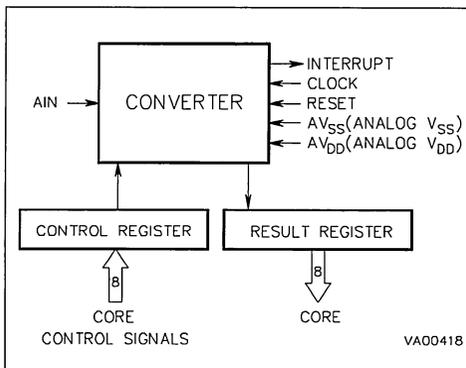
Figure 36. A/D Converter Control Register
