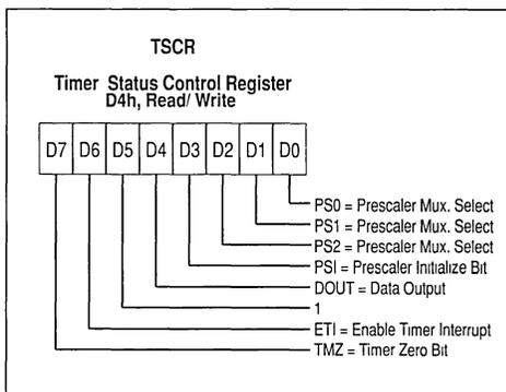
Figure 28. Timer Working Principle
