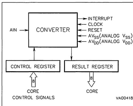
Figure 36. A/D Converter Control Register
