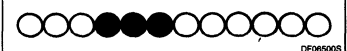
NOTE: The strands of one turn are indicated by black dots. Figure 25. A Multiple-Wire Winding of 4 Turns, Each of 3 Strands
