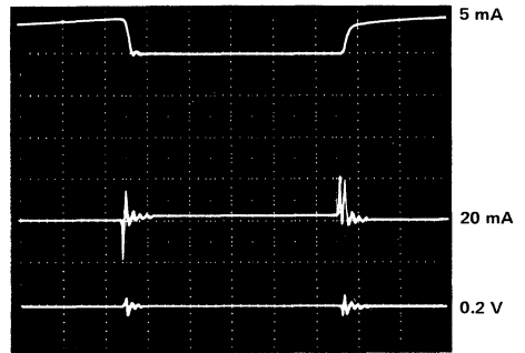
d) SN74LS00 load: C_L = 50 \text{ pF}
