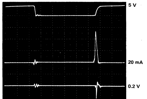
l) SN74ALS1000A load: C_L = 50 \text{ pF}
