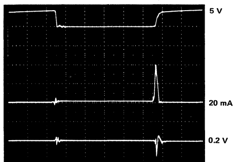
j) SN74ALS00A load: C_L = 50 \text{ pF}
