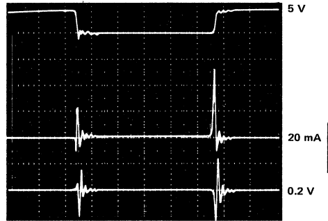
f) SN74AS00 load: C_L = 50 \text{ pF}
