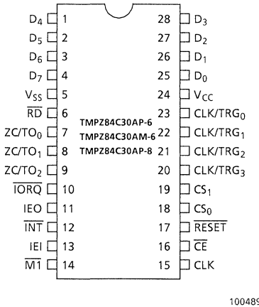
Figure 2.1 DIP, SOP Pin Connections
