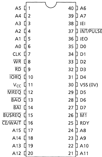
Figure 2.1 DIP, SOP Pin Assignments
