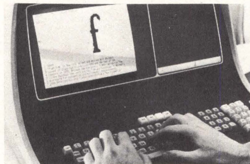
A magnified picture of the character as it appears on the page along with several lines of surrounding text for context can be displayed on the CRT for operator verification or correction of ambiguous letters
