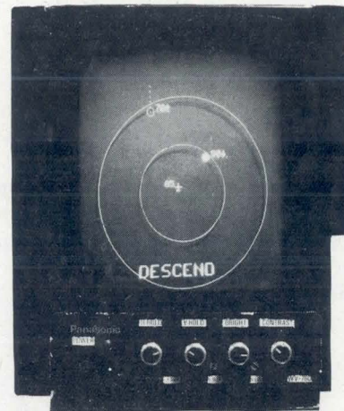
Fig 4 CRT display. Combining symbols and alphanumeric in a graphical presentation, display is heading oriented and centered on the aircraft to simulate pilot's view through windshield. Small aircraft symbol represents simulator. Solid ring shows intruder at 1 o'clock, less than 3 mi away heading toward simulator, and descending through 9000 ft. Ring of dots shows still another aircraft at 11 o'clock, 5.5 mi away, heading toward simulator and climbing through 7000 ft
