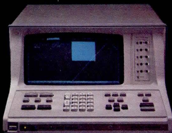
Hewlett-Packard 1610B A sophisticated data-domain-only logic analyzer
