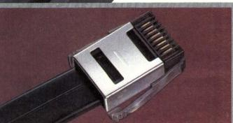
Shielded Data Link connectors available in 4, 8, 16, 24 contact configurations. Insulation-displacing design provides redundant contact on each conductor. Built-in polarization/keying system.
