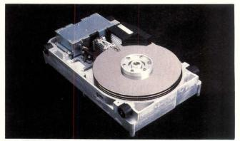
Capacities of 500 Mbytes are attained by Priam's 8-in. Winchesters. To pack six disks into the drive, a staggered arrangement is used with the 3370 type heads. Two heads are mounted side by side on the actuator. One reads the bottom surface of the upper disk; the other, the top surface of the lower disk.
