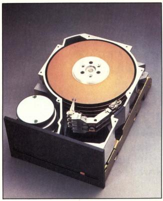
An 80-Mbyte capacity, 51/4-in. drive, Computer Memories' CM7880 writes data on four platters. The ability to pack platters into the compact unit results from mechanical design and use of 3370-type head flexures.
