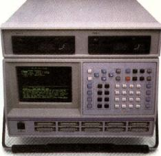
The K105-D gives you two levels of HELP at the touch of a button. First, step-by-step operating instructions that appear along the bottom of the analyzer screen. Second, a menu that allows you to select more detailed "help" should you need it.
