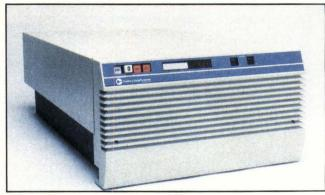
Using 19 thin-film heads to read/write on five 14-in. platters, Century Data's Advanced Marksman Series 571 meets high capacity, high performance needs. Multiple heads/platter cuts average access time to 19 ms.
