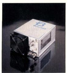
A single output switcher, the 1000-W HL1000 fits the standard 5- x 8- x 11-in. format. Pin-out compatibility provides several control features including supply paralleling, advance thermal warning, power fail detect, remote sense output status, and remote inhibit.
