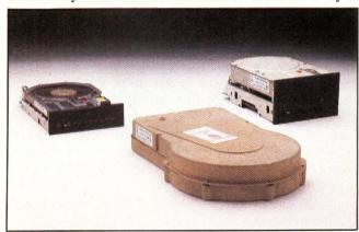
Sizes of standard 51/4-in. full-height (rear left) and halfheight (rear right) are compared with that of half-height 8-in. package (foreground). Seagate's 8-in. half-height ST8100 stores 100 Mbytes. The height of the package allows all control electronics to fit with the drive in a standard fullheight form factor.
