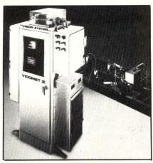
Featuring a 640 x 485 matrix array, the Vidomet IIE is capable of 256 levels of contrast. Its image processor can operate at the high speed data handling rates necessary for current online inspection tasks. Up to 32 separate cameras, either solid state or Vidicon type, can connect to a single system. Applications include line gauging of dimensional measurements, parts identification, or feature verification at production line speeds. Penn Video Inc, 929 Sweitzer Ave, Akron, OH 44311. Circle 277
