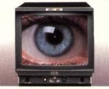
Barco provides a full range of color dis-plays, from 14" to 26," with horizontal scanning systems from 15 to 37.5 Khz, and vertical scanning from 40 to 120 Hz. Choose between standard and high resolution (0.31 dot triad pitch) CRT's with normal and long persistence phos-phors, available in both delta gun and the most advanced in-line gun technology. And, of course, Barco is expert at manufacturing to your own specifications and requirements.
