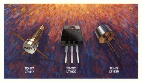
Our new bipolar high resolution transistors come in three packages: TO-39 (LT1839), TO-117 (LT1817), and TO-220 (LT1820). These new transistors are priced in the \$4 to \$8 range in small quantities.
