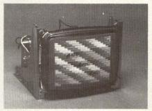
Model 14DD981 color terminal has a 14-in. CRT with a 90-degree reflection angle. The noninterlaced resolution of 720 dots x 396 lines, has a usable display of 210 x 280 mm. The terminal provides a 25-MHz video bandwidth, 24.5-kV high voltage, and 15.75-kHz horizontal scanning frequency. AC power input is 120 V  $\pm 10$  percent at 60 Hz, or 240 V ± 10 percent at 50 Hz. It weighs 27.5 lb, and provides 16 display colors. Audiotronics, 7428 Bellaire Ave, N Hollywood, CA 91605.
