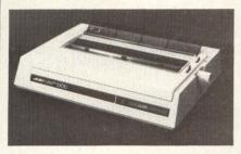
Low cost, high speed daisy wheel printer 6300 has 96 chars and operates at 40 chars/s with a 60 dBA noise level. A 16-in. platen and multistrike ribbon round out special features. Operating on a Centronics parallel or RS-232-C serial interface, power consumption is 70 W. A 3-Kbyte buffer memory is expandable to 15 Kbytes. The printer measures 600 x 400 x 125 mm, and weighs 14 kg. Juki America, 299 Market St., Saddle Brook, NJ 07662.
