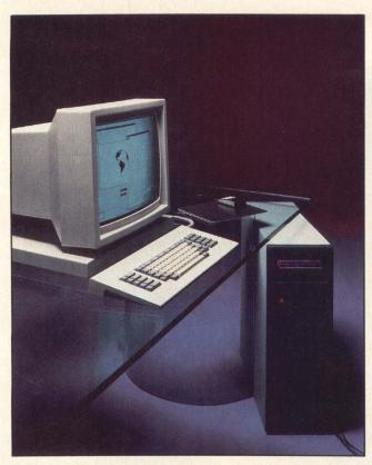
As with other standalone workstations, the Sun-2 family runs on a Unix derivative that allows each station to operate without a separate disk storage unit. Instead, diskless nodes use the Ethernet network to perform demand paging as well as routine file 1/0. The 68010-based workstation is designed for easy upgrading to true 32-bit computing power when the 32-bit (both address and data) 68020 chips become available.
