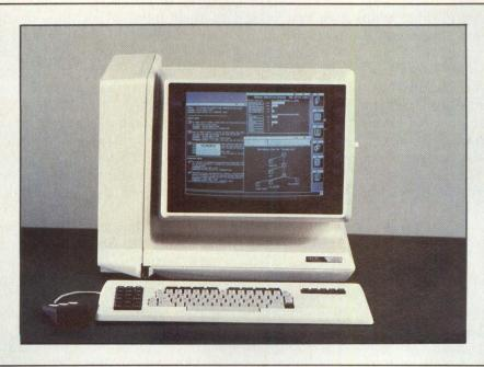
The Apollo DN320 workstation distinguishes itself by incorporating a standard hardware floating point processor. The processor is implemented in bit-slice technology. This allows structuring of both 32-and 64-bit floating point data formats that adhere to the IEEE standard. As another node in the Domain network, the DN320 offers each user 1.5 Mbytes of main memory, 16 Mbytes of virtual address space and a 1024- x 800-pixel display. A 68010 is used as the central processor.
