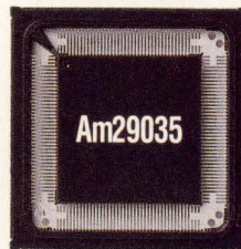
32-bit RISC processor with 4K cache and programmable bus sizing.
