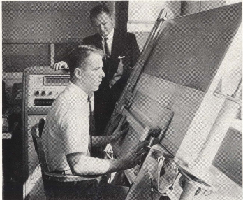
Moving the cursor arm over points on the chart, the operator closes a foot switch to record coordinates and all identifying codes automatically on punched cards or paper tape.
