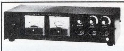
The triple model 1301 consists of a fixed 5-Vdc supply at 1 A and two 0.5-A, 5- to 18-Vdc, continuously adjustable supplies. The three outputs can operate independently or connect in series or parallel to provide up to 18 Vdc at 1 A or up to 41 Vdc at 0.5 A. Features include a front-panel ammeter (1 A full scale) and voltmeter (20 Vdc full scale). Current limiting protects against short circuits and overloads. **Global Specialties Corp**, 70 Fulton Terr, PO Box 1942, New Haven, CT 06509.
