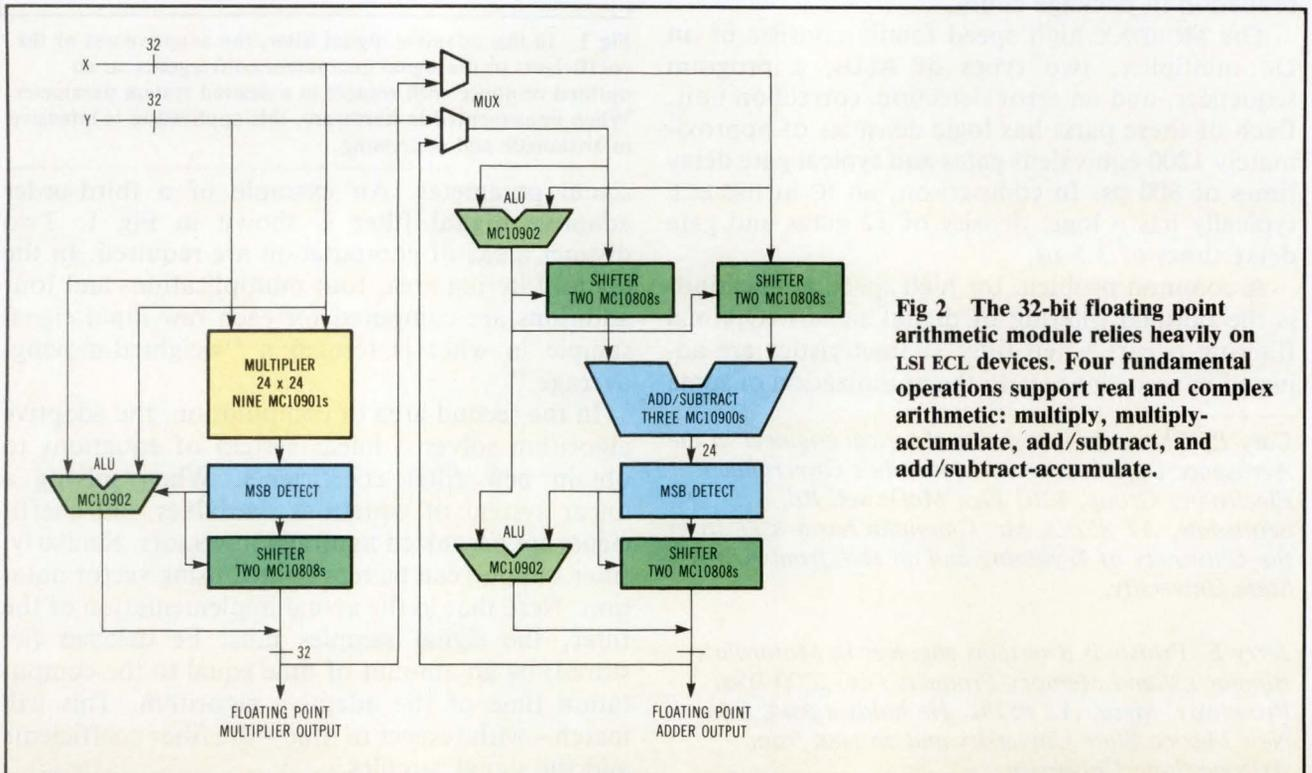
**Fig 2** The 32-bit floating point arithmetic module relies heavily on LSI ECL devices. Four fundamental operations support real and complex arithmetic: multiply, multiply-accumulate, add/subtract, and add/subtract-accumulate.
