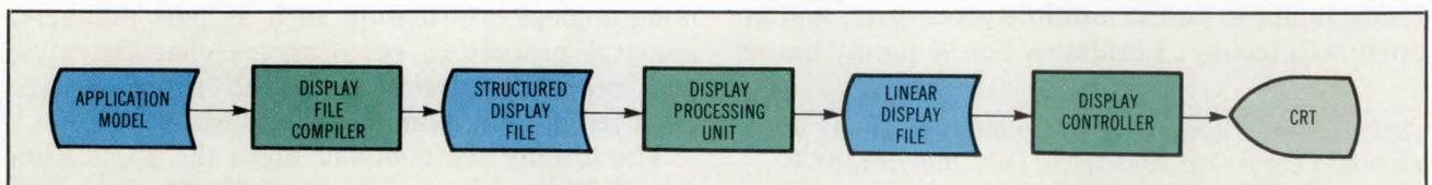
Fig 1 An interactive graphics system can be modeled by means of the GDP. All the parts of this linear, conceptual model need not be implemented in separate modules, but the functionality is usually present somewhere.
