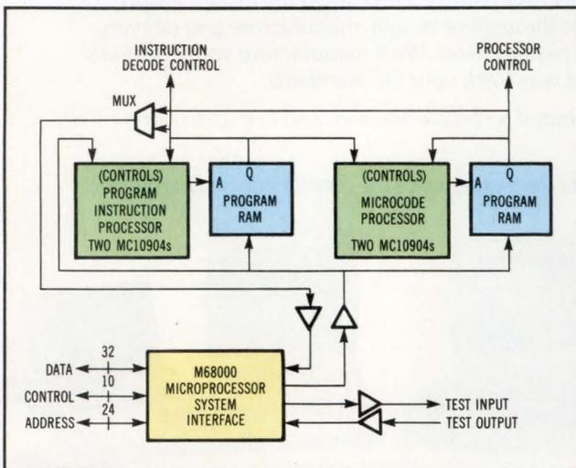
**Fig 5** The LSI ECL computer is configured as an attached coprocessor to an executive host (ie, M68000), allowing several to be controlled. The MC10904 is used as the program sequencer for the instructions and the microcode control.
