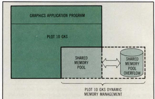
**Fig 4** A dynamic memory management facility exists in PLOT 10's GKS and allows allocation and reuse of a memory pool. When the pool is full, parts are copied to a disk file. The parts copied are intelligently chosen for minimal system impact.
