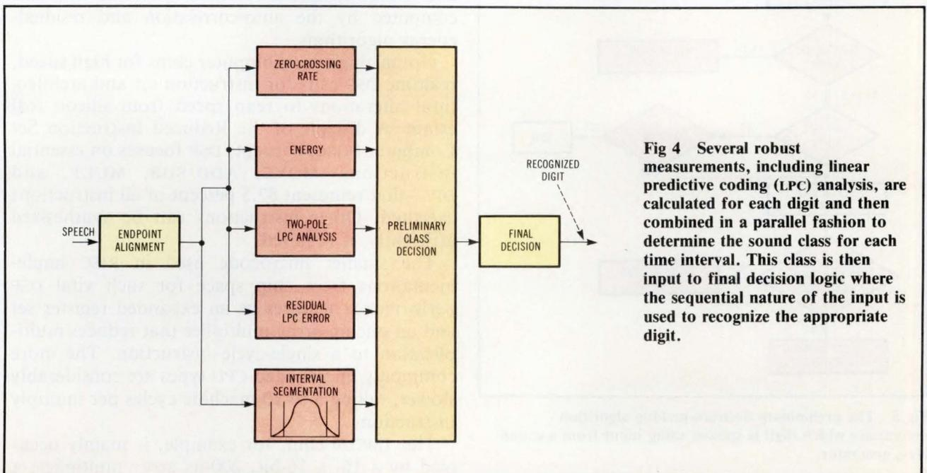
**Fig 4** Several robust measurements, including linear predictive coding (LPC) analysis, are calculated for each digit and then combined in a parallel fashion to determine the sound class for each time interval. This class is then input to final decision logic where the sequential nature of the input is used to recognize the appropriate digit.
