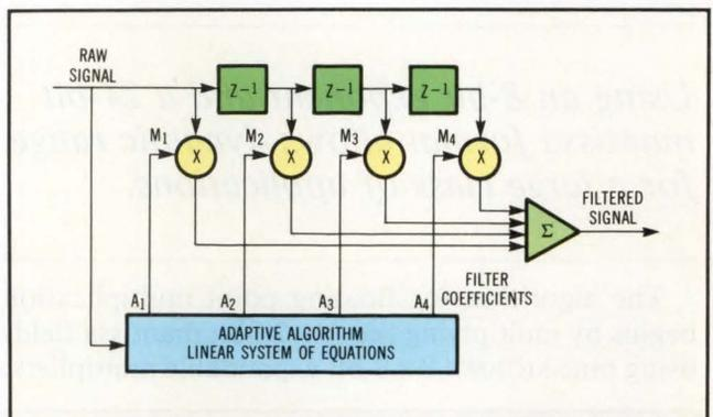
**Fig 1** In this adaptive digital filter, the adaptiveness of the coefficients to the signal guarantees convergence to an optimal response with respect to a desired system parameter. When implemented in hardware, this application is intensive in arithmetic and addressing.
