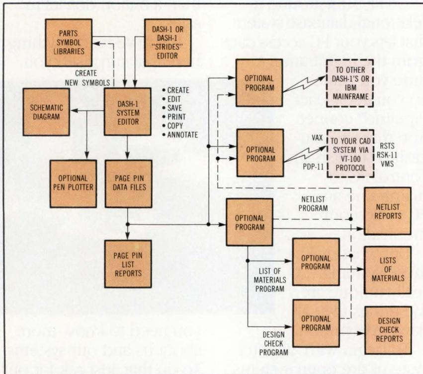
Personal computer-based CAD systems like DASH-1 from FutureNet Corp do not limit designers to what can fit on their desktops. Communication packages link the personal computer to mainframe or minicomputers, or to expensive peripherals like plotters and printers. Database extraction also allows list of materials, engineering change orders, and design rule checking to be performed.
