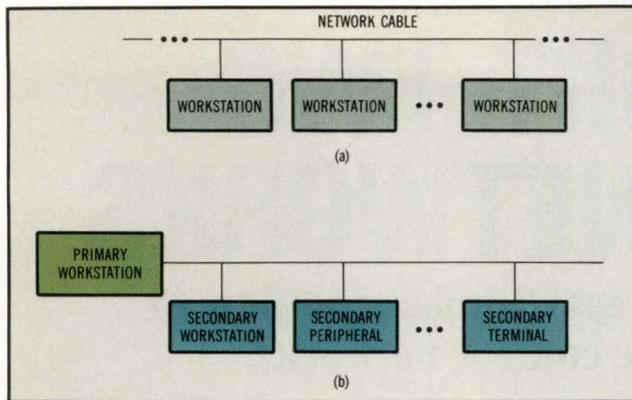
**Fig 1** A multidrop configuration is the simplest means of network expansion (a). Additional stations are connected directly to the network cable, but some addressing method must be used to avoid party-line reception by all stations. HDLC/SDLC protocols provide a controlled-access technique where a primary station controls all bus access and determines which secondary stations respond to its commands (b).
