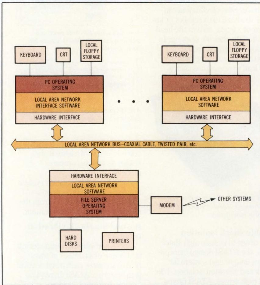
**In a general bus-oriented net, such as 10-Net or NetWare, individual PCs transfer files over a bus via a combination of hardware and software. One or more stations can serve as file or print servers.**
