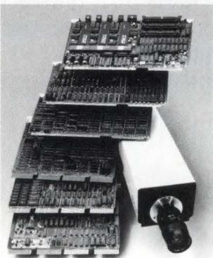
The modules contain programmable I/O Transformation Tables and provide for B&W and RGB output for full color processing.
