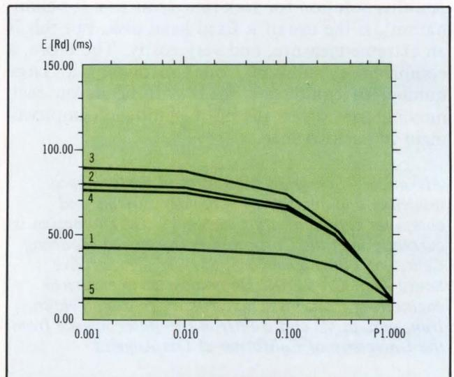
Fig 1 Computer analysis produces mean disk response times of five disk organizations. Plots of disk times converge at the fastest response time—when the probability of no arm movement equals 1.
