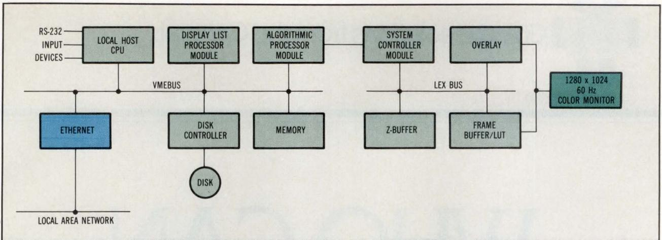
**Fig 4** In this architecture, the display system supports workstation design with a range of options for both the GDP and the 32-bit VMEbus-based open system architecture. The hardware options take care of medium and high resolution graphics designs.
