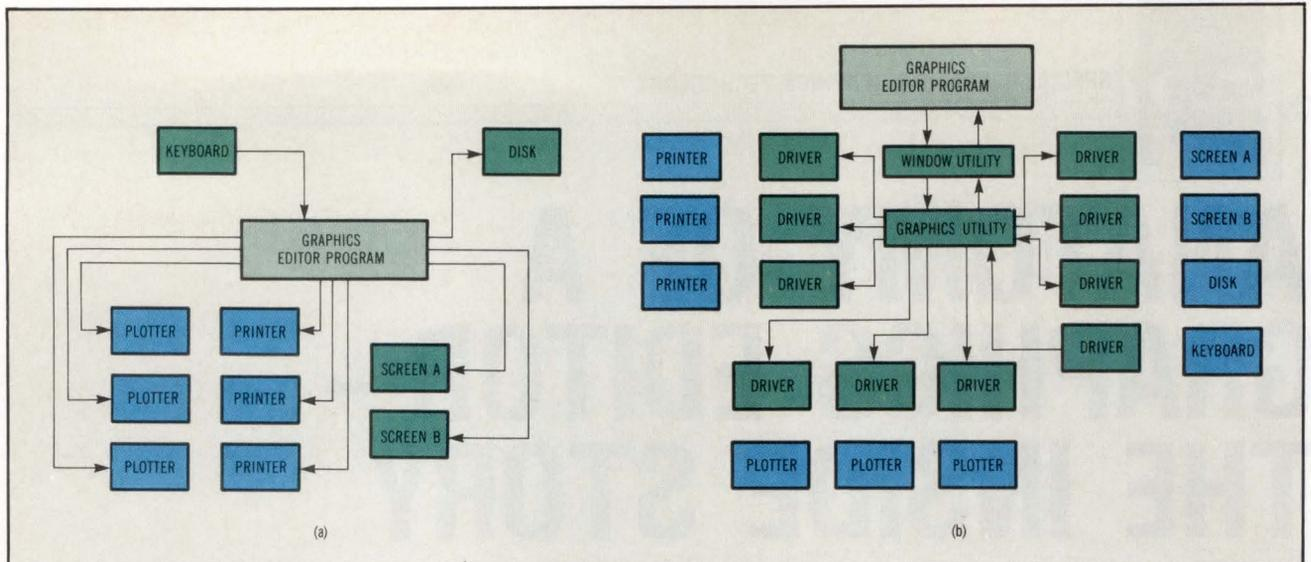
**Fig 1** The Sound Presentations graphics editor can be developed from the ground up (a), or with the aid of a graphics tool kit (b). Tools allow a faster time-to-market while custom design offers only incremental technology advantages.
