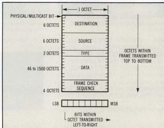
**Fig 3** Each Ethernet frame consists of five fields. Destination and source fields indicate where the message is going and from which station it originated. The data field can contain as few as 46 bytes of data and as many as 1500.
