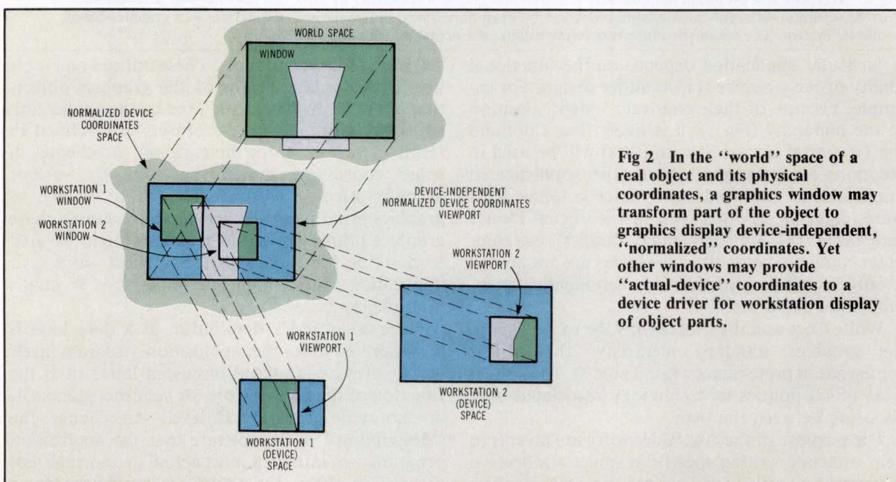
**Fig 2** In the "world" space of a real object and its physical coordinates, a graphics window may transform part of the object to graphics display device-independent, "normalized" coordinates. Yet other windows may provide "actual-device" coordinates to a device driver for workstation display of object parts.
