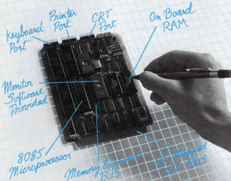
**Cubit's new I/O Processor controls a CRT, printer and keyboard.**
