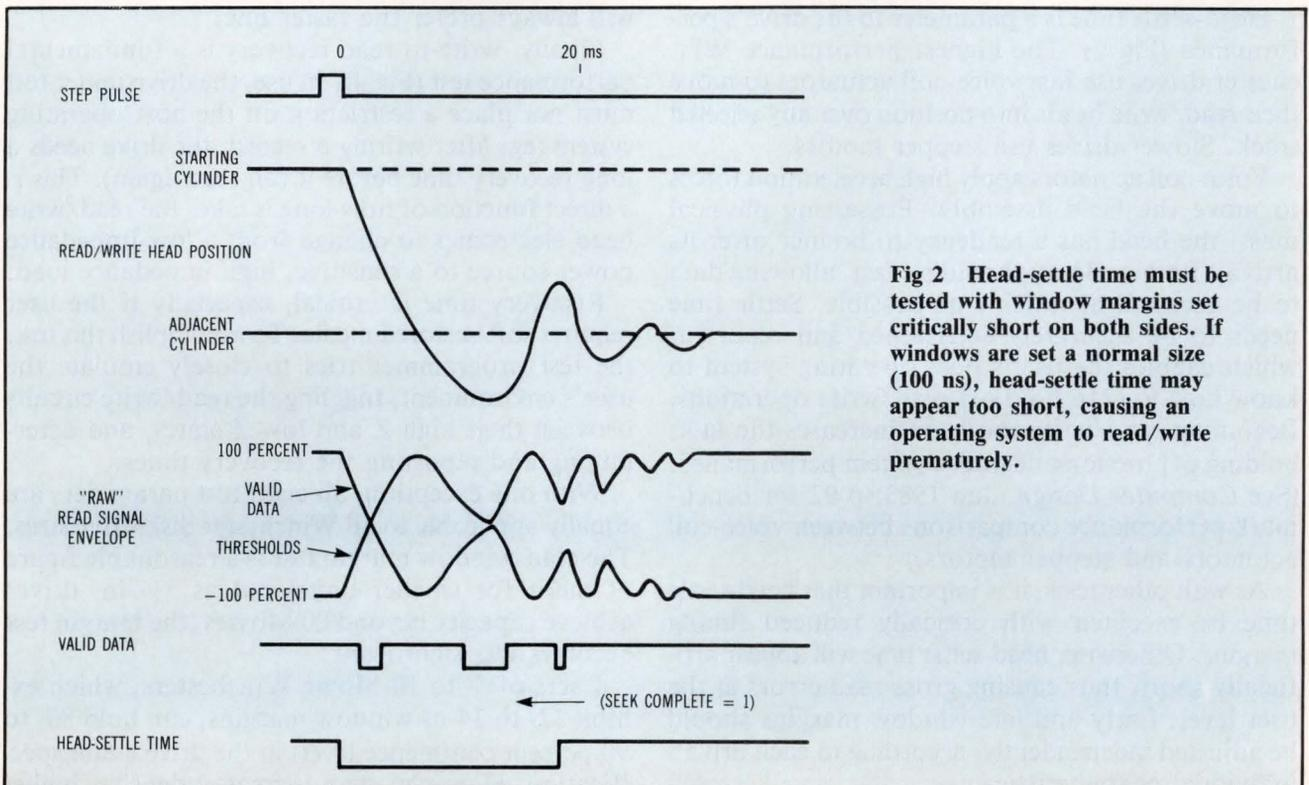
**Fig 2** Head-settle time must be tested with window margins set critically short on both sides. If windows are set a normal size (100 ns), head-settle time may appear too short, causing an operating system to read/write prematurely.
