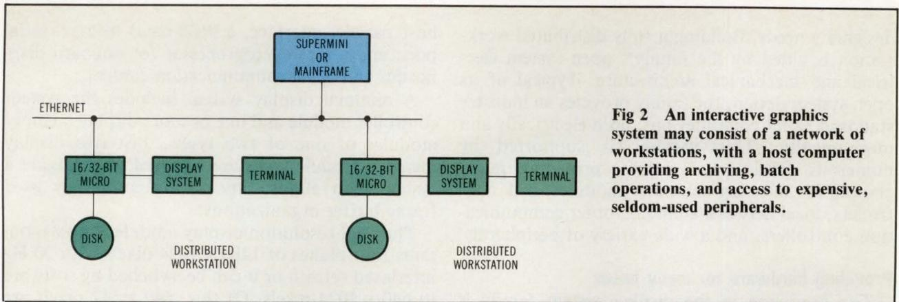
**Fig 2** An interactive graphics system may consist of a network of workstations, with a host computer providing archiving, batch operations, and access to expensive, seldom-used peripherals.
