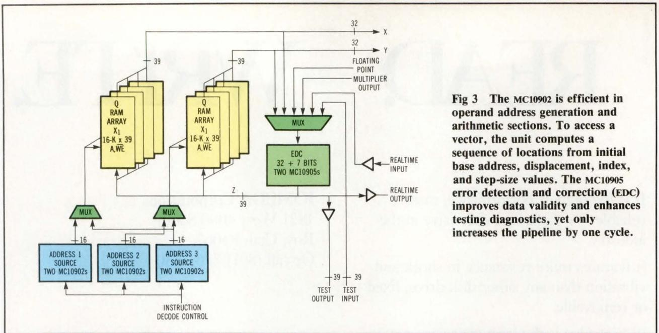
**Fig 3** The MC10902 is efficient in operand address generation and arithmetic sections. To access a vector, the unit computes a sequence of locations from initial base address, displacement, index, and step-size values. The MC10905 error detection and correction (EDC) improves data validity and enhances testing diagnostics, yet only increases the pipeline by one cycle.
