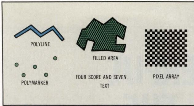
**Fig 1** The primitives or basic drawing functions in the Graphical Kernel System (GKS) standard are limited to the five capabilities shown. As the GKS is designed, these may be called in a program through standard Fortran language binding.
