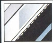
An aluminum layer between the shadow mask and the screen reflects light from the phosphor dots out toward the viewer and at the same time prevents errant screen light from reaching the photodetector.
