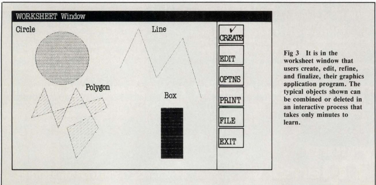
Fig 3 It is in the worksheet window that users create, edit, refine, and finalize, their graphics application program. The typical objects shown can be combined or deleted in an interactive process that takes only minutes to learn.
