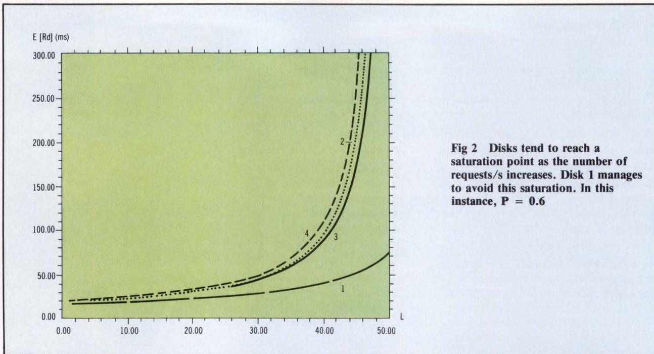
**Fig 2** Disks tend to reach a saturation point as the number of requests/s increases. Disk 1 manages to avoid this saturation. In this instance,  $P = 0.6$
