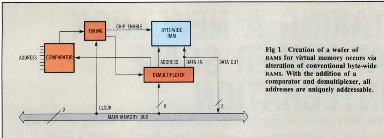
**Fig 1** Creation of a wafer of RAMs for virtual memory occurs via alteration of conventional byte-wide RAMs. With the addition of a comparator and demultiplexer, all addresses are uniquely addressable.
