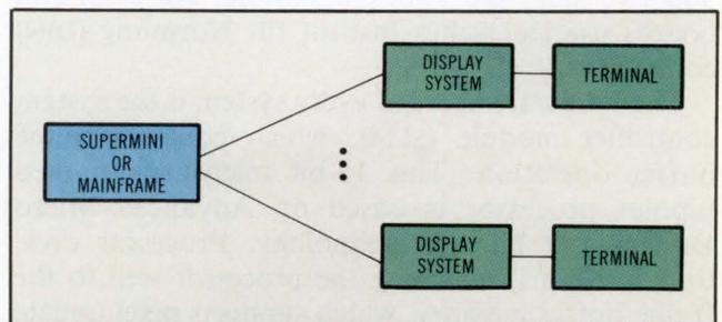
**Fig 3** Open system architecture supports host-controlled graphics, distributed network graphics, or a partially distributed system architecture in which major portions of the graphics display pipeline are off-loaded from the host computer.
