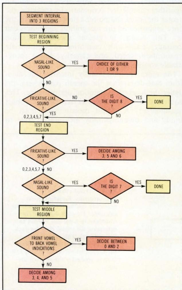
**Fig 5** The preliminary decision-making algorithm determines which digit is spoken using input from a sound class generator.
