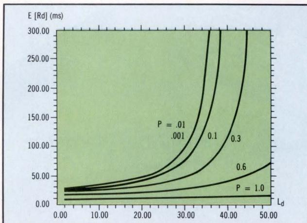
**Fig 3** As the probability of disk arm movement increases, mean response time also increases. These increased times are justified by cost trade-offs of this organization (for suitable values of  $P$ ).
