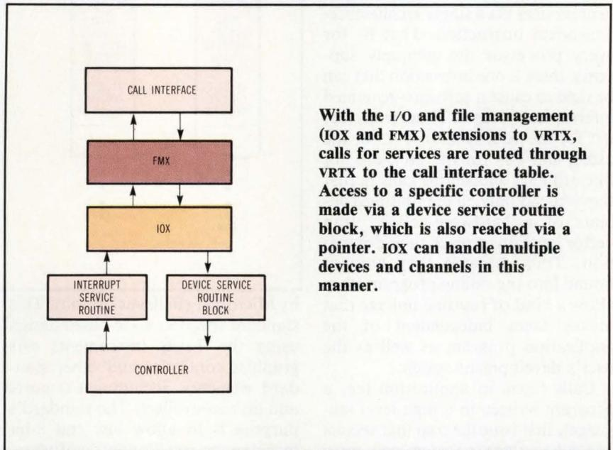
**With the I/O and file management (IOX and FMX) extensions to VRTX, calls for services are routed through VRTX to the call interface table. Access to a specific controller is made via a device service routine block, which is also reached via a pointer. IOX can handle multiple devices and channels in this manner.**
