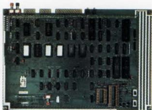
Add only a power supply and terminal for an instant system. Evaluate and program the HMOS MC68705 (M68705EVM and MC1468705 (M1468705EVM) Series MCUs. As low as a super \$495.00 price.
