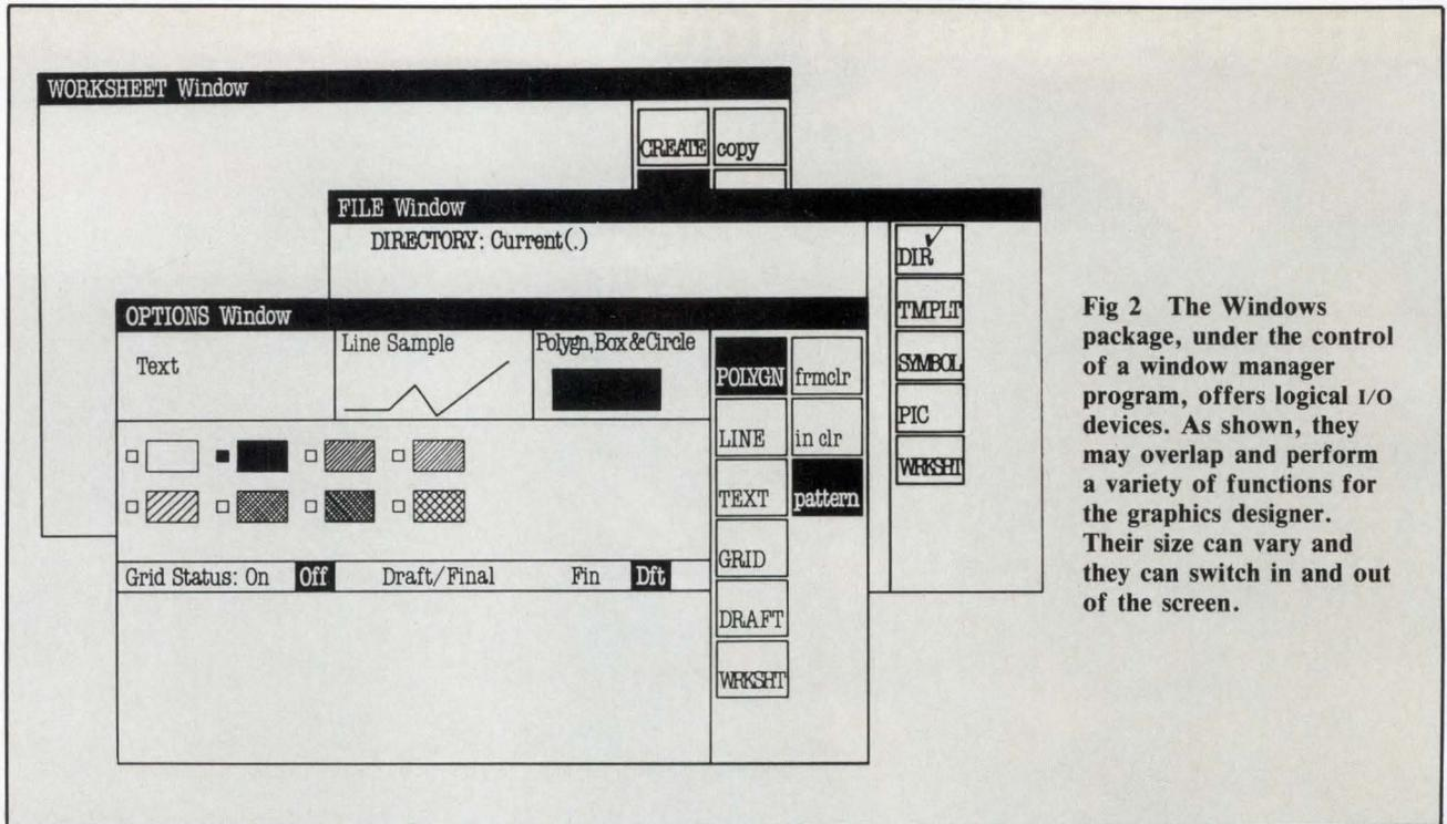
Fig 2 The Windows package, under the control of a window manager program, offers logical I/O devices. As shown, they may overlap and perform a variety of functions for the graphics designer. Their size can vary and they can switch in and out of the screen.
