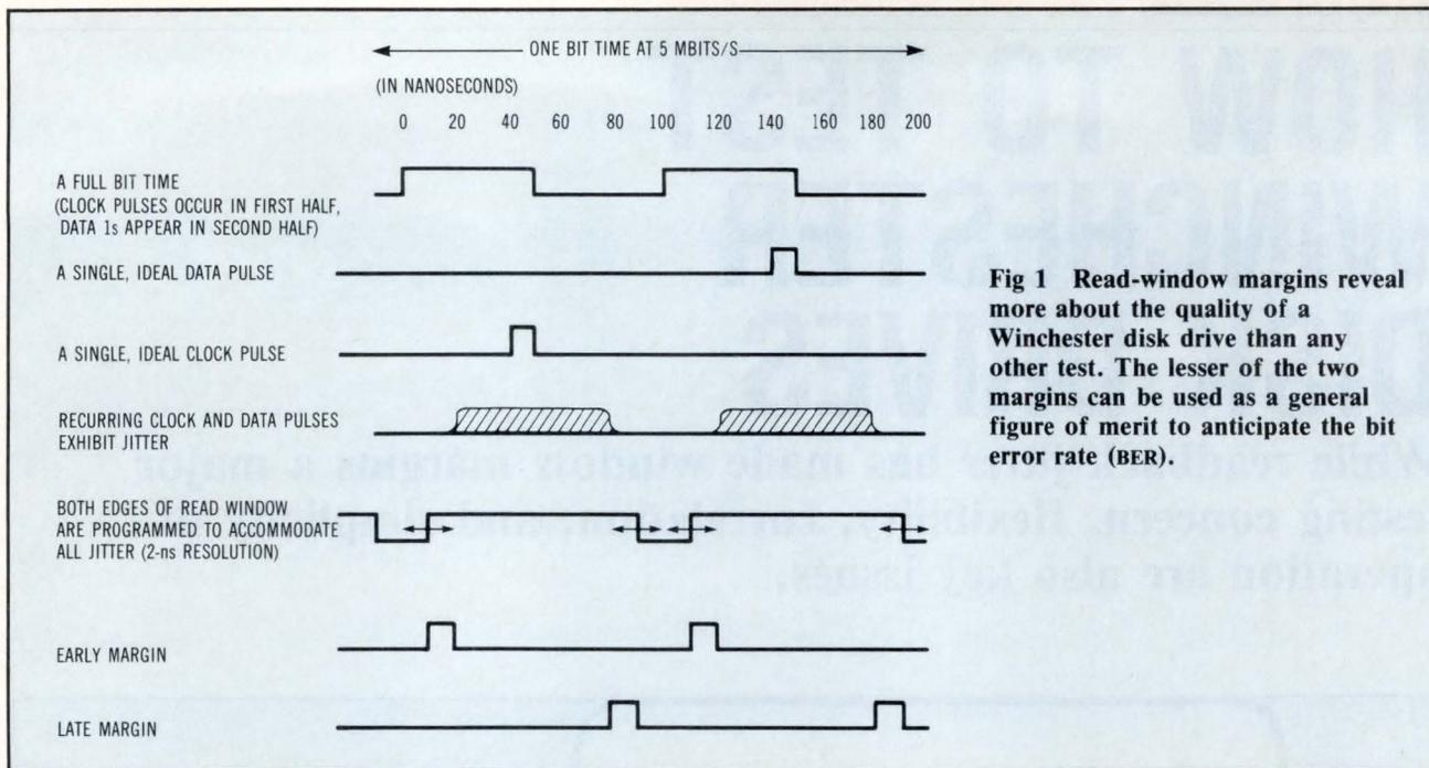
**Fig 1 Read-window margins reveal more about the quality of a Winchester disk drive than any other test. The lesser of the two margins can be used as a general figure of merit to anticipate the bit error rate (BER).**
