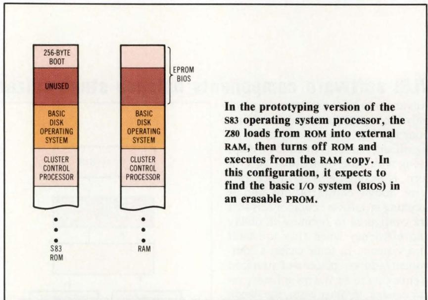
**In the prototyping version of the S83 operating system processor, the Z80 loads from ROM into external RAM, then turns off ROM and executes from the RAM copy. In this configuration, it expects to find the basic I/O system (BIOS) in an erasable PROM.**
