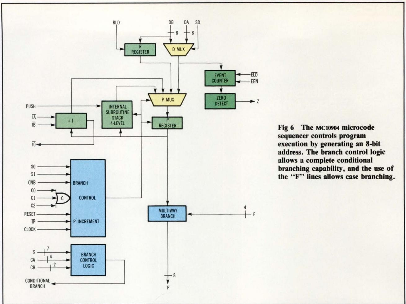
**Fig 6** The MC10904 microcode sequencer controls program execution by generating an 8-bit address. The branch control logic allows a complete conditional branching capability, and the use of the "F" lines allows case branching.
