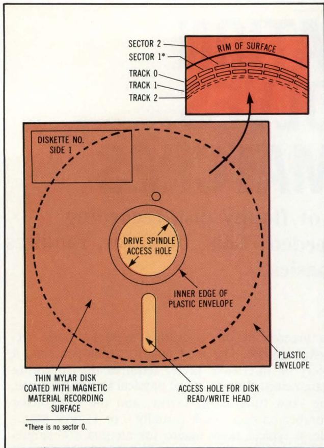
**Fig 1** The IBM 3740 format for 8-in. diskettes consists of 77 tracks arranged in 26 sectors of 128 bytes each. To improve throughput efficiency, the sectors are skewed (interleaved) by a given factor, such as 6. The starting sector (0 or 1) coincides with the index mark.
