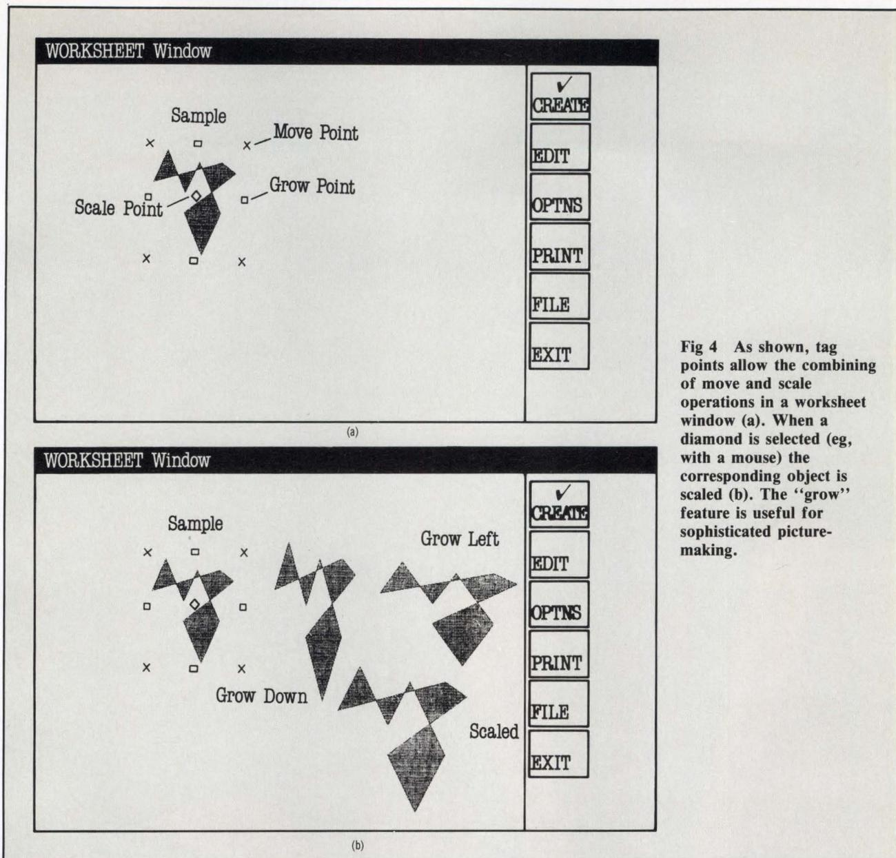
Fig 4 As shown, tag points allow the combining of move and scale operations in a worksheet window (a). When a diamond is selected (eg, with a mouse) the corresponding object is scaled (b). The "grow" feature is useful for sophisticated picture-making.
