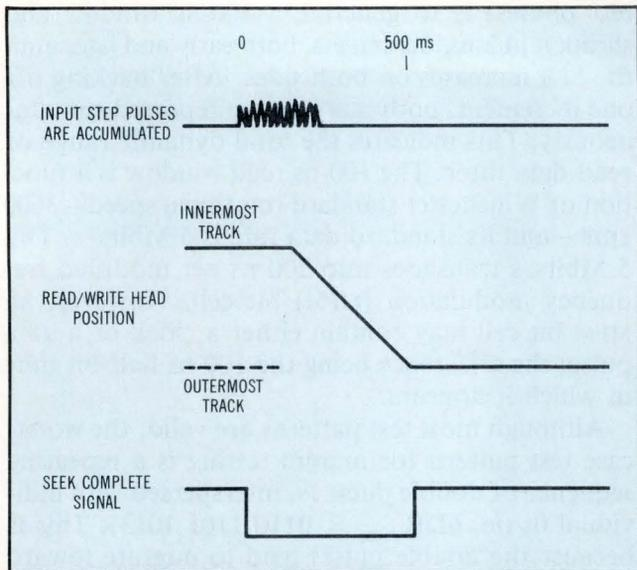
**Fig 3** Access time is a performance test for smart Winchester drives featuring a buffered-step mode. The test involves the sum of the step-pulse input string duration plus lateral head motion. Manufacturers typically specify only head motion.
