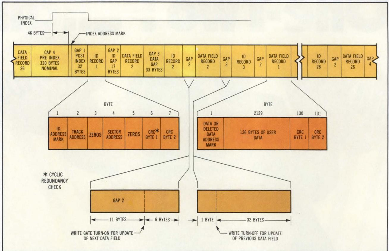
**Fig 2 To format a diskette to the IBM 3740 scheme (128 bytes per sector) with a Western Digital controller, a Write command must be issued and the data register loaded with the following: the sector size in bytes, the number of sectors per track, the number of usable tracks, the identification address mark, the side number, the gap sizes, and the step rate.**
