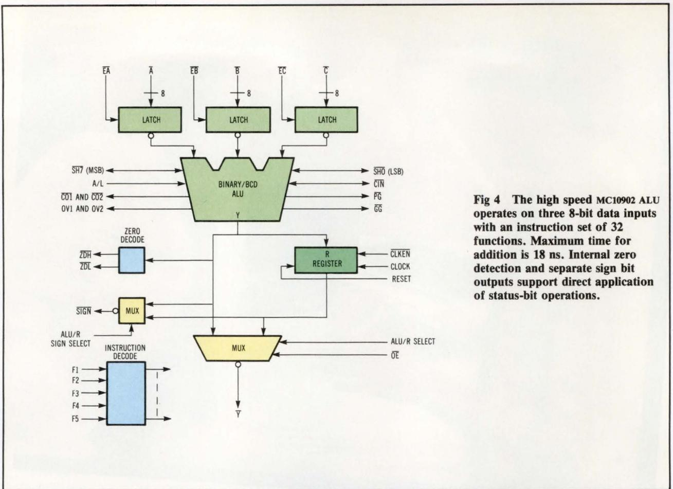
**Fig 4** The high speed MC10902 ALU operates on three 8-bit data inputs with an instruction set of 32 functions. Maximum time for addition is 18 ns. Internal zero detection and separate sign bit outputs support direct application of status-bit operations.
