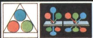
Delta configuration of the electron guns helps maintain both high resolution and optimum spot profile throughout the screen — not just the center.
