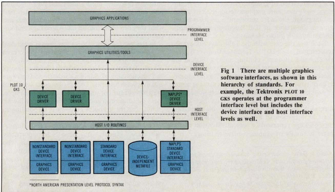
**Fig 1** There are multiple graphics software interfaces, as shown in this hierarchy of standards. For example, the Tektronix PLOT 10 GKS operates at the programmer interface level but includes the device interface and host interface levels as well.
