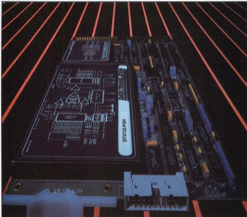
driven. Setting the DMA and Done interrupt bits through software selects the DMA mode. Up to 64 Kwords can be transferred without program intervention. After 64 Kwords, the process must be restarted.
