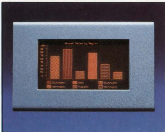
Using patented self-scan with memory, the model 120 flat panel combines the inherent memory of ac plasma with the powerful addressing of dc plasma to reduce expensive driver electronics. The result is a full-page display, with 480- x 250-pixel graphics and 80-col x 25-row alphanumeric, that promises to compete price-wise with high quality CRT moni-
