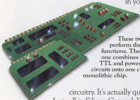
These two boards perform the same functions. The smaller one combines several TTL and power driver circuits onto one custom monolithic chip.
