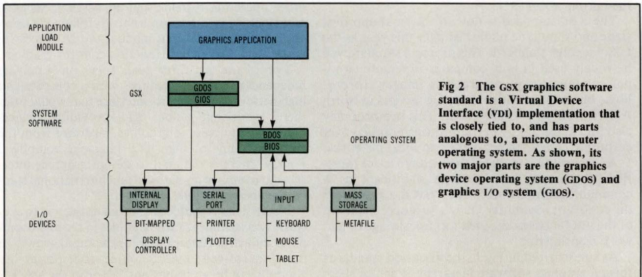
**Fig 2** The GSX graphics software standard is a Virtual Device Interface (VDI) implementation that is closely tied to, and has parts analogous to, a microcomputer operating system. As shown, its two major parts are the graphics device operating system (GDOS) and graphics I/O system (GIOS).
