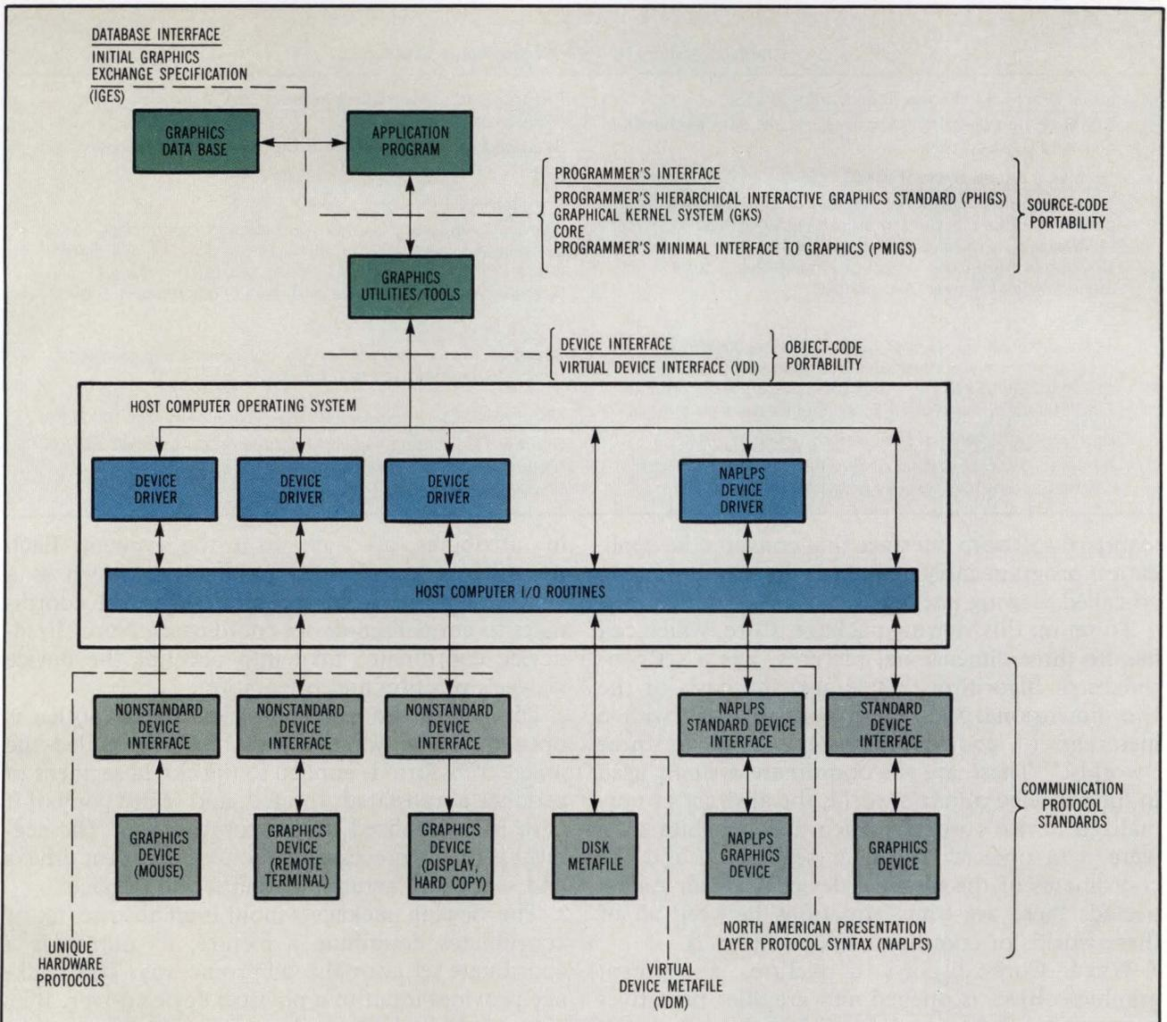
**Fig 1 Accepted and proposed national and international graphics standards all have carefully defined software to provide separate, different-functionality interfaces between data bases, programmers, and devices in a graphics-based computer system. The schematic represents relationships, not actual positioning.**
