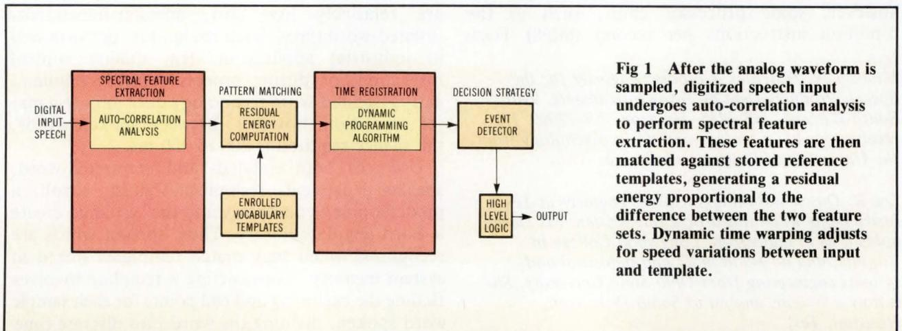
**Fig 1** After the analog waveform is sampled, digitized speech input undergoes auto-correlation analysis to perform spectral feature extraction. These features are then matched against stored reference templates, generating a residual energy proportional to the difference between the two feature sets. Dynamic time warping adjusts for speed variations between input and template.
