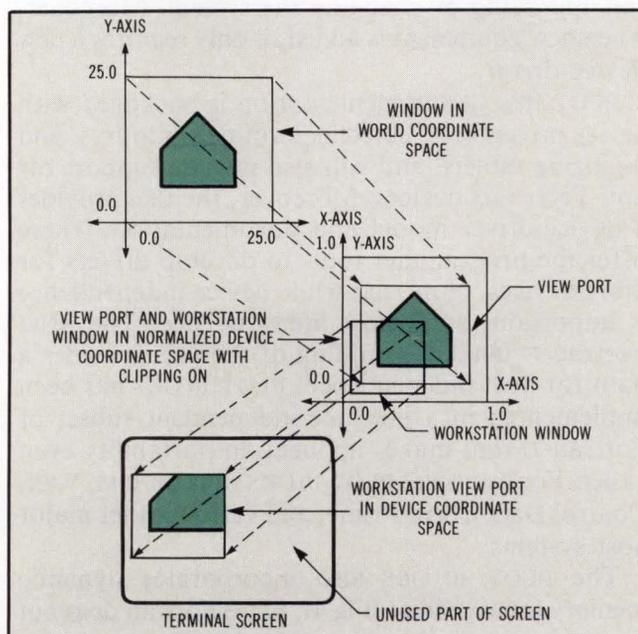
**Fig 3** The GKS allows multiple window-view port transformations at a terminal screen. This feature allows scaled drawings and the use of a rectangular screen without restricting graphics to a square area.
