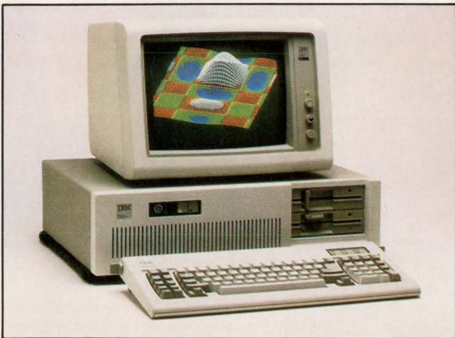
The IBM PC offers a variety of high performance graphics I/O devices. One of these is the Professional Graphics Controller and Display. It can draw up to 256 colors concurrently from a palette of 4096 colors.
