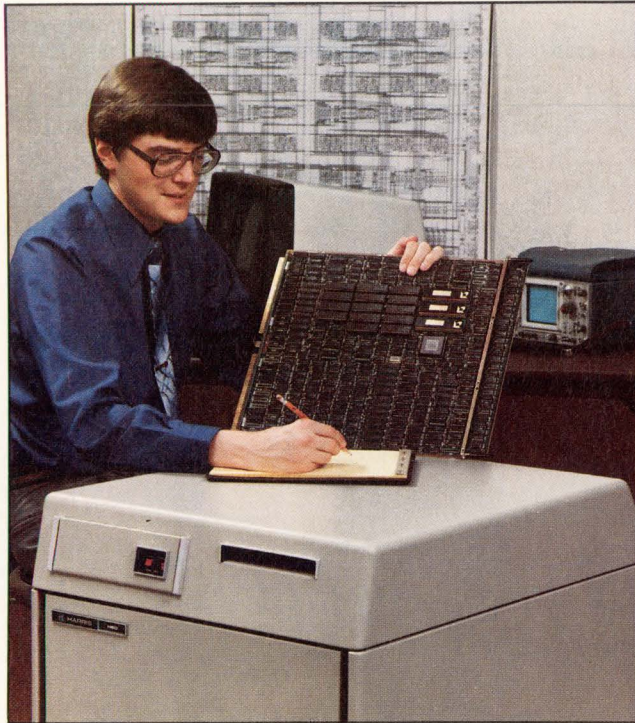
Harris 60 uses VLSI/LSI circuits and custom gate arrays that have over 8000 gates each. These, along with 256-Kbit RAMs used in the memory system, decrease bulk and cut costs.
