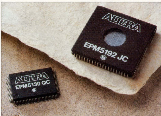
The 84-pin, UV-erasable EPM-5192JC MAX programmable logic device from Altera, in a windowed, ceramic J-lead chip carrier, has 192 macrocells and 7,500 gates. The EPM5130QC MAX part, in a one-time programmable plastic quad flatpack, pushes PLD pin counts to 100.
