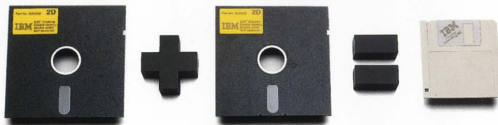
It takes two 360KB 5¼" diskettes to hold as much as one 720KB 3½" diskette.
