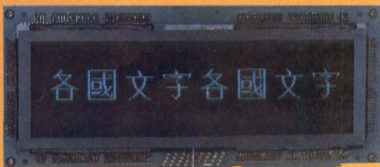
Vacuum Fluorescent Module, super fast bit mapped display. 256 x 64 pixels.
