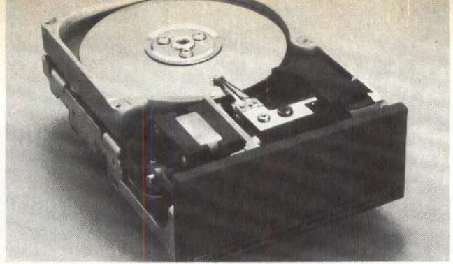
Figure 5: Miniscribe's new sub-4" Winchester stores over 200 Mbytes of formatted data.
