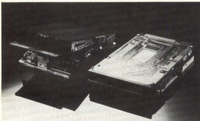
Figure 1: Citizen offers their slim, 1" high microfloppy drive in a top-load configuration.
