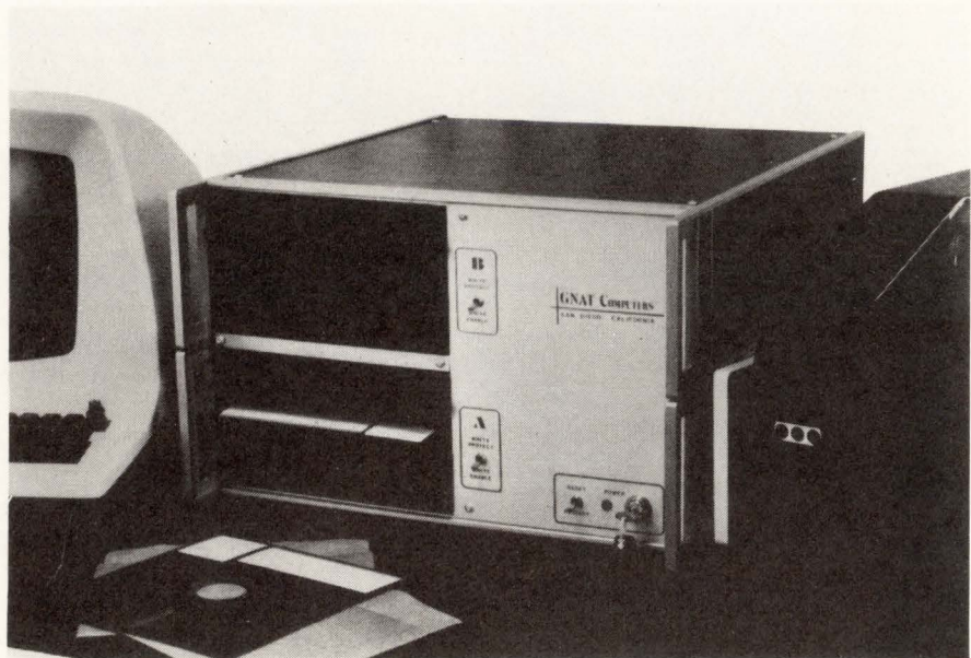
Fig 2 The Gnat floppy disk microcomputer, an 8080-based computer and development system from Gnat Computers, San Diego, CA.
