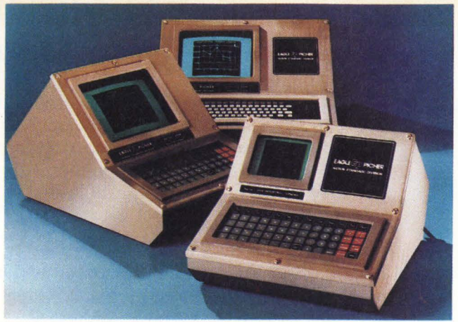
Figure 2: Integral display screen and membrane keyboard with letters in alphabetic order make Eagle-Picher's FacTer terminals well-suited to the industrial environment.
