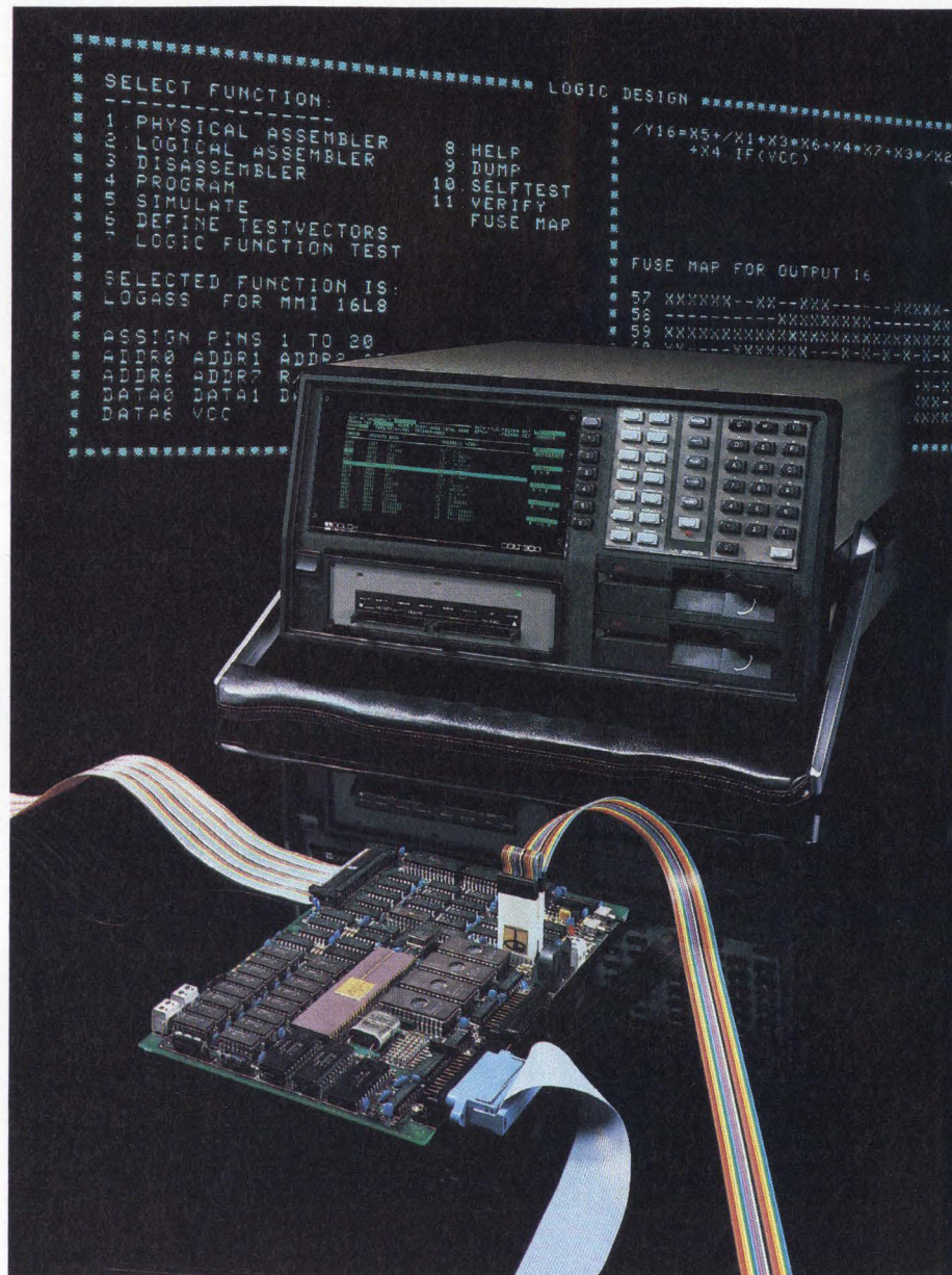
Figure 1: The COLT 300 from Dolch can function as either a portable or benchtop development system.
