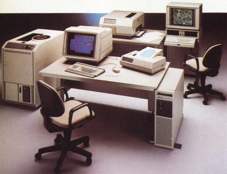
Tektronix 6200 Series Intelligent Graphics Workstations use multiple 32-bit CPUs. The 6212 Workstation with a 6000 family display in the foreground is connected to the Tektronix 4115B Display Terminal with 4691 color graphics copier support and to the 4695 color graphics copier. The cabinet at right houses two 300 Mbyte SMD disk drives and a 9-track tape drive.
