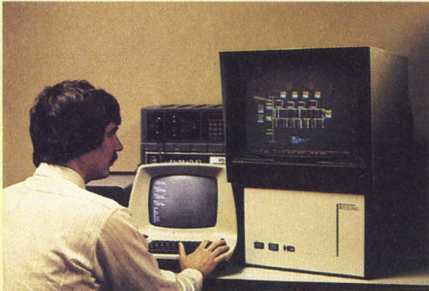
Figure 1: RTCS on the right is testing a control program running on the Allen-Bradley PLC-3 programmable controller.
