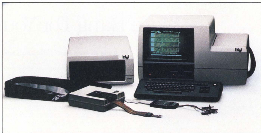
Figure 4: Intel's bond-out technology gives the I 2 ICE system special access to internal processor states that are virtually inaccessible in any other way. The result is a near Intel monopoly on emulators for the 8051 microcontroller and the 80286 microprocessor.
