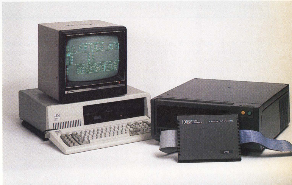
Figure 2: Kontron's Development Adapter enables an IBM Personal Computer to host their slave emulator subsystem.
