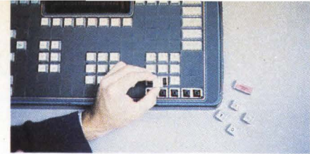
Figure 7: Processes being controlled are generally unique, and this Flexus keyboard kit from USData provides total user configurability of 155 keys; even the legends on the keycaps are chosen or created by the system designer.
