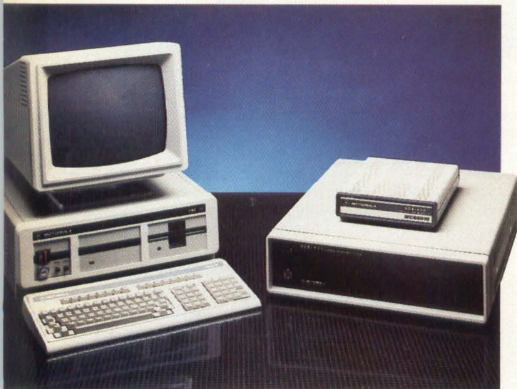
Figure 2: Motorola Microsystems supports full 16-bit development with its VME/10 computer and the HDS-400 hardware development station. Besides hardware debugging, the company is incorporating state analysis.
