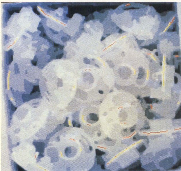
Figure 5: Cyto IV three-dimensional image of a bin containing parts to be picked out by robot arm. Vertical relief was pseudocolored from processed data collected by laser range finding.
