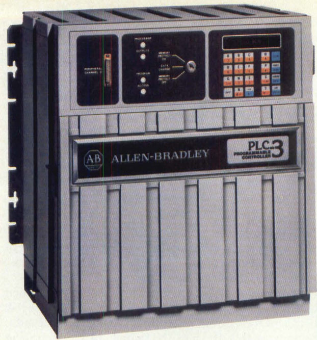
Figure 3: The Allen-Bradley PLC-3 is one of the largest programmable controller systems available, controlling up to 8196 I/O points with up to 1.92 Mbytes of memory. Basic programming provides computer functions like floating point math and report generation.
