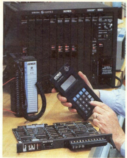
Figure 1: The GENIUS I/O System from General Electric consists of an I/O block, bus controller module and hand-held monitor. Aimed at applications requiring 100 or more I/O points, it can be placed up to 2000 feet from the programmable controller.
