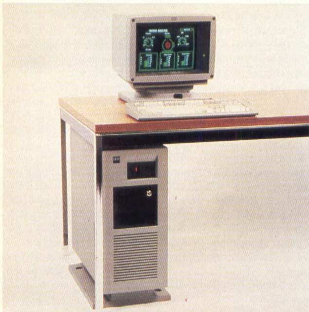
Figure 2: The 7531 industrial computer from IBM is a factory hardened version of its PC/AT. Standard equipment includes 512 Kbytes of memory, a 1.2 Mbyte diskette drive and seven available I/O expansion slots.
