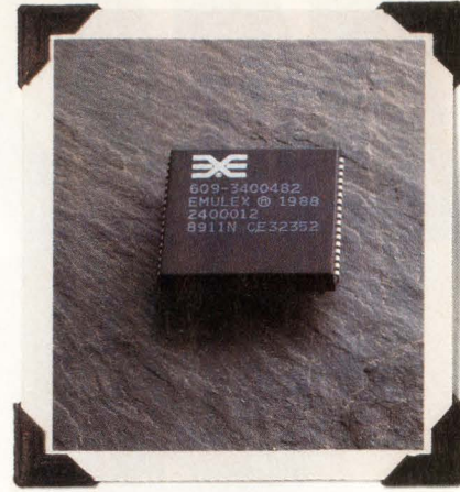
1988-ESP200. Second generation SCSI arrives with SCSI-2 support and Parity Pass-through.
