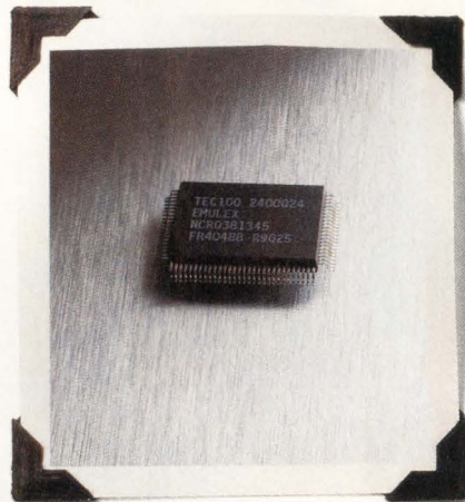
1989-TEC100. EMD combines disk, buffer, and SCSI controllers in a single chip.
