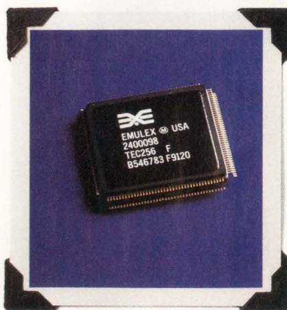
1991-TEC256. The first Fast and Wide SCSI disk controller also boasts the fastest disk data rate and highest system bandwidth.
