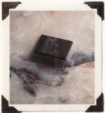
1990-FAS236. We deliver the first Fast SCSI chips with a 16-bit DMA port.
