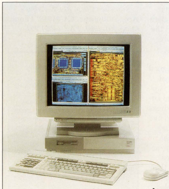
Extending the low end of its RISC-based workstation line, Hewlett-Packard's Series 9000 Model 710 runs at almost 50 SPECmarks.
