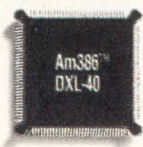
The 40MHz DXL-40 and the 33MHz SXL-33 are available in low-cost PQFP packaging.
